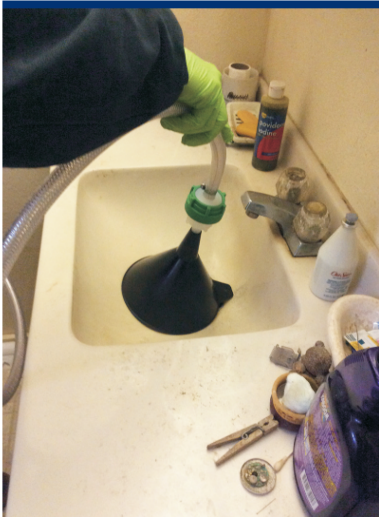
Photo 19 Mercury vapor screening inside the bathroom of the primary residence after replacing P-trap.
