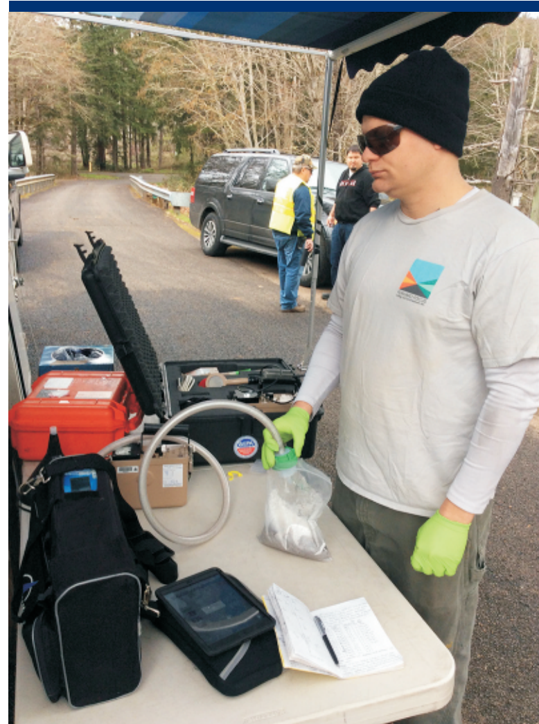
Photo 20 Mercury vapor screening of ex-situ soil from the excavated area after heating in accordance with EPA Region 10 Mercury Response Module.
