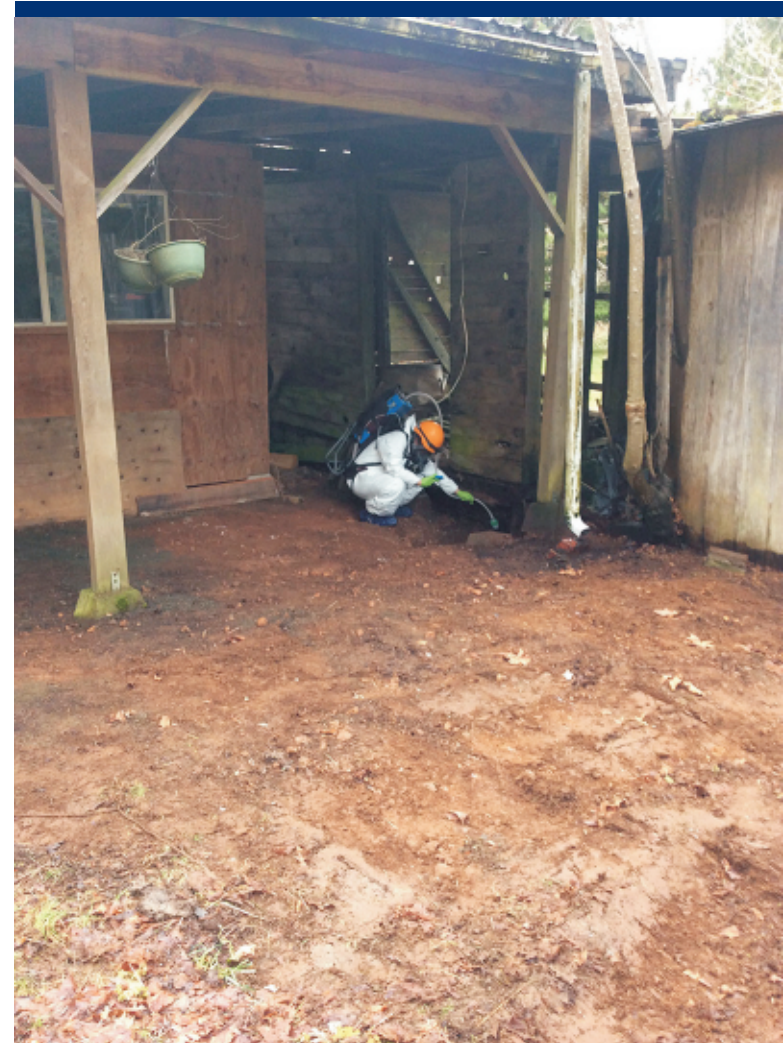
Photo 9 Screening excavated areas with the Lumex mercury vapor analyzer.
