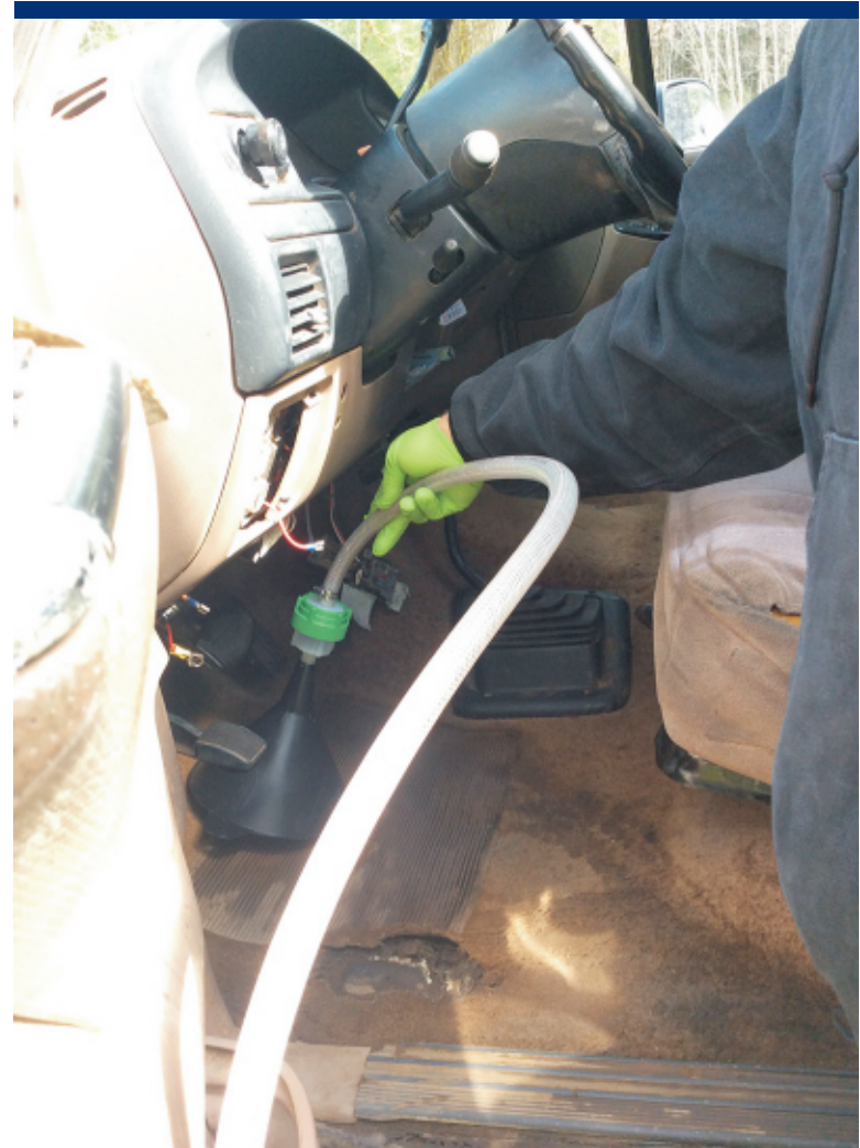
Photo 14 Screening the interior of the truck for mercury vapors.
