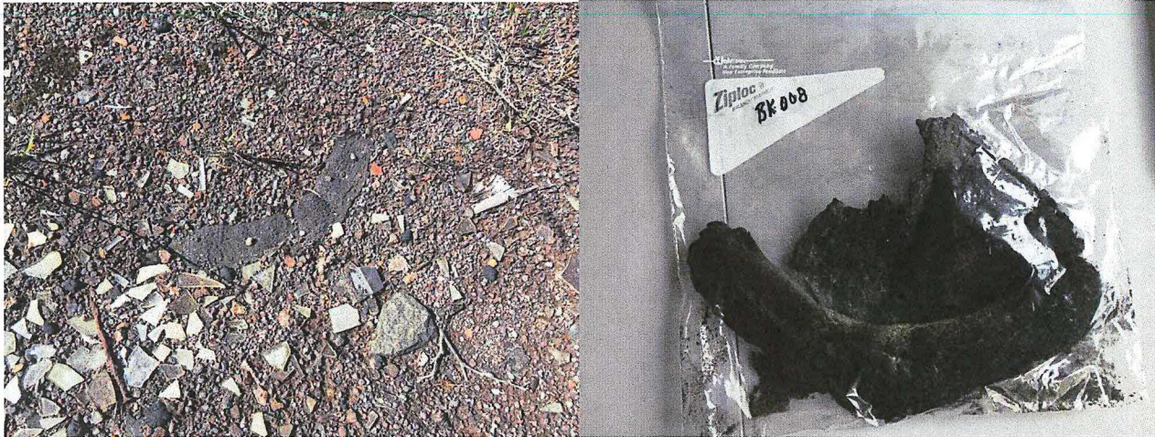
Asbestos Containing Material (ACM) found throughout the site.
