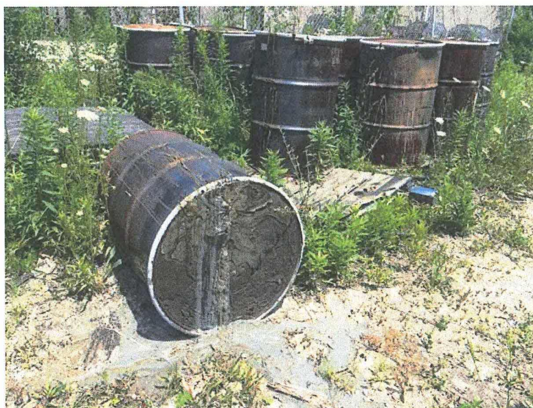
Photo 6: Leaking drum with stained soil, VOCs = 440 ppm, Flashpoint = 96 °F
