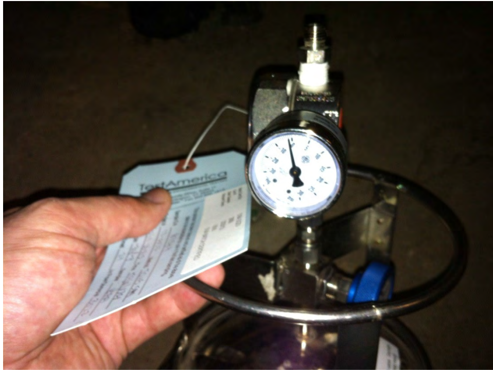
Photograph 7: RST 2 noted the vacuum reading on the pressure gauge before stopping Sample No. P008-SG001-130312-01 on March 13, 2013.
