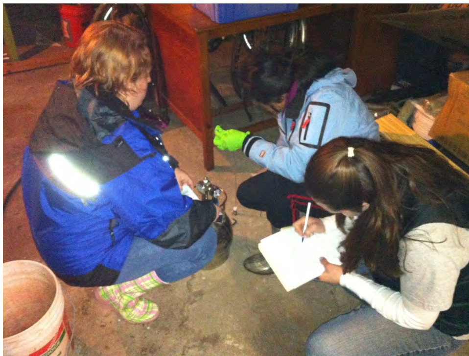
Photograph 5: RST 2 and EPA DESA personnel install inlet tubing for sub-slab soil gas sampling and record start time and initial vacuum pressure of the Summa canister on March 12, 2013.
