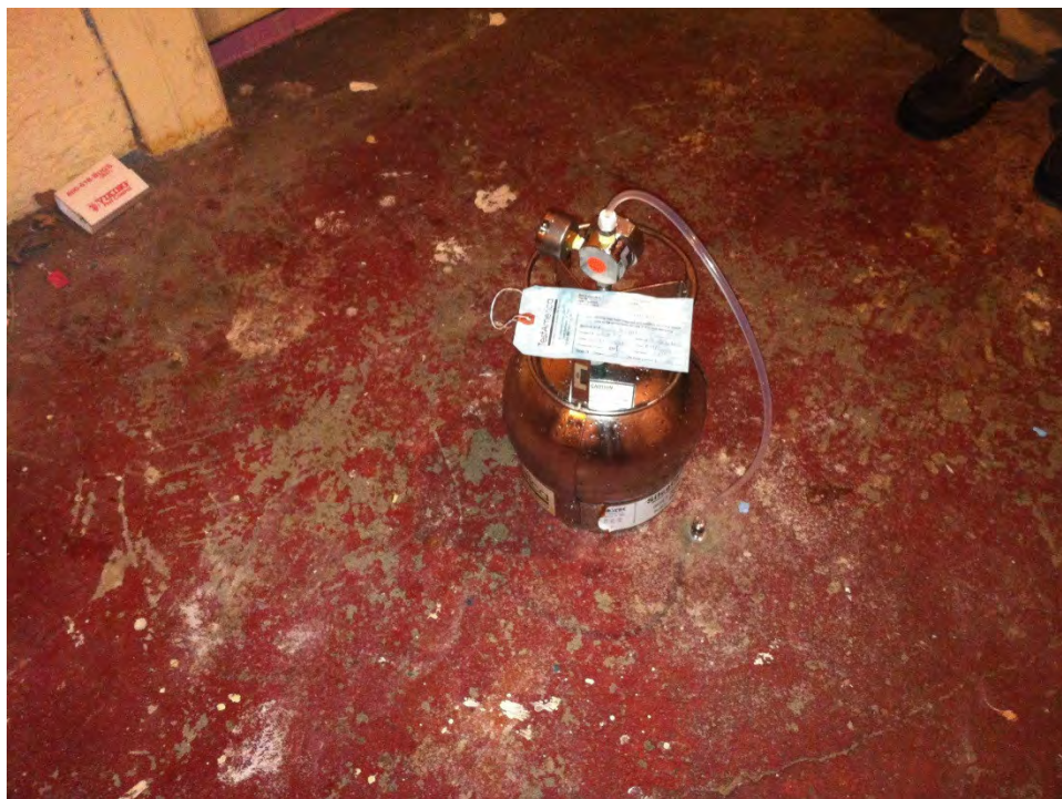
Photograph 9: View of Summa canister deployed at sample location P010-SG001 on March 12, 2013.
