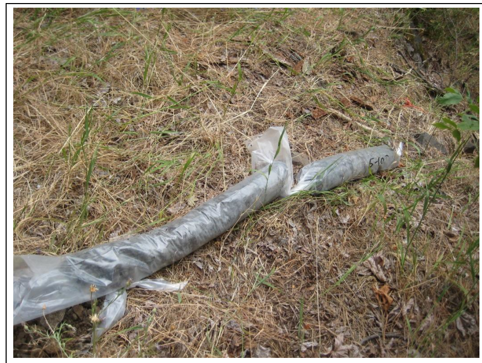
Photograph 15. Well drilling cuttings were placed in plastic sleeves and marked with depth. Cultural monitors were given the opportunity to cut open the bag and sort through the excavated material.
