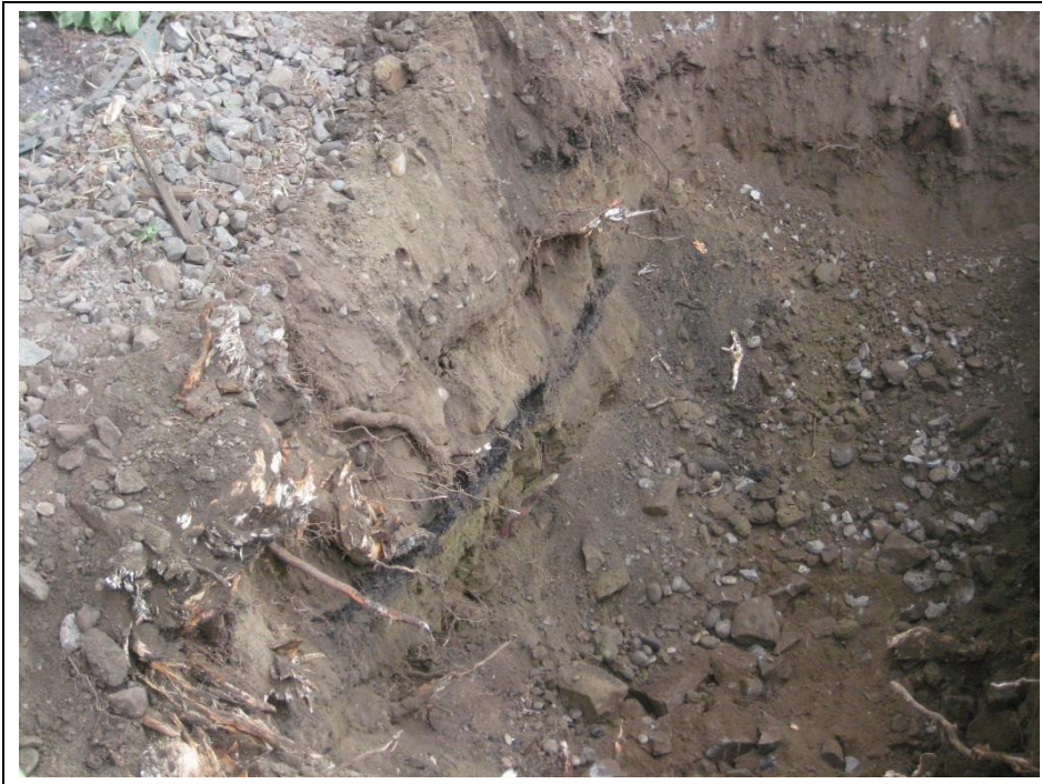
Photograph 4. Sidewall of pothole excavation shown. A thin layer of coal waste associated with the railroad is visible in the sidewall. This layer was observed throughout the excavation. Aspect: southwest.
