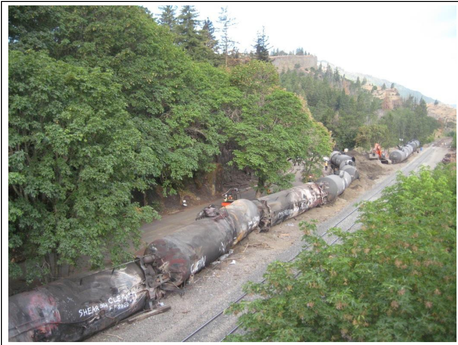
Photograph 1. Overview of derailment area after rail cars have been purged, cleaned, and prepared for transport offsite. The excavator in the background is stockpiling material bladed from the southern side of the railroad. Photograph taken from the overpass. Aspect: southwest.
