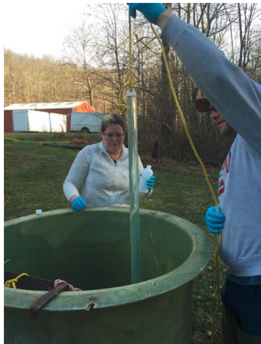
Photo No. IMG_3138; Taken on 12/09/15 at 14:02 hours by START-ET. Facing South. TechLaw scientists using a bailer to collect a sample from the primary sump location.
