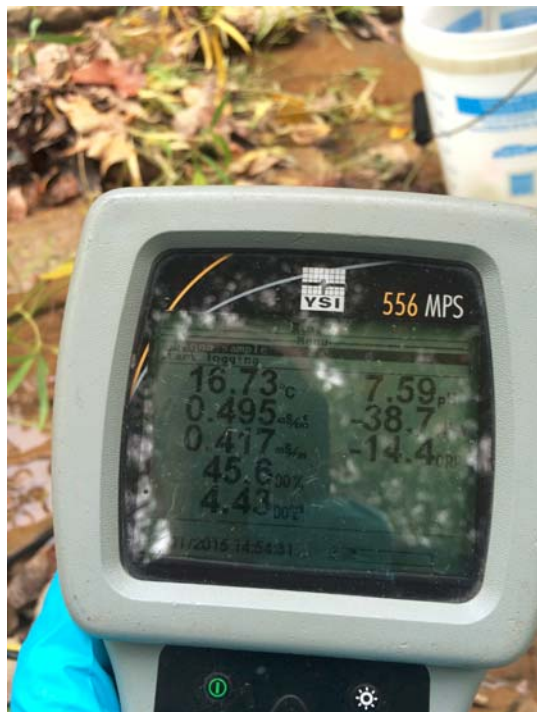
Photo No. IMG_0424; Taken on 10/01/15 at 14:59 hours by START-MG. Facing Down. Water Quality Readings at WG-PW-006.
