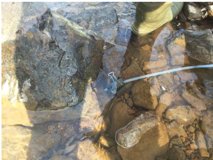
Photo No. IMG_3125; Taken on 12/09/15 at 12:26 hours by START-JW. Facing Down. The set up used by TechLaw to collect samples from the bottom of the water column at sample WG-SW-0017/dup WG-SW-0018.
