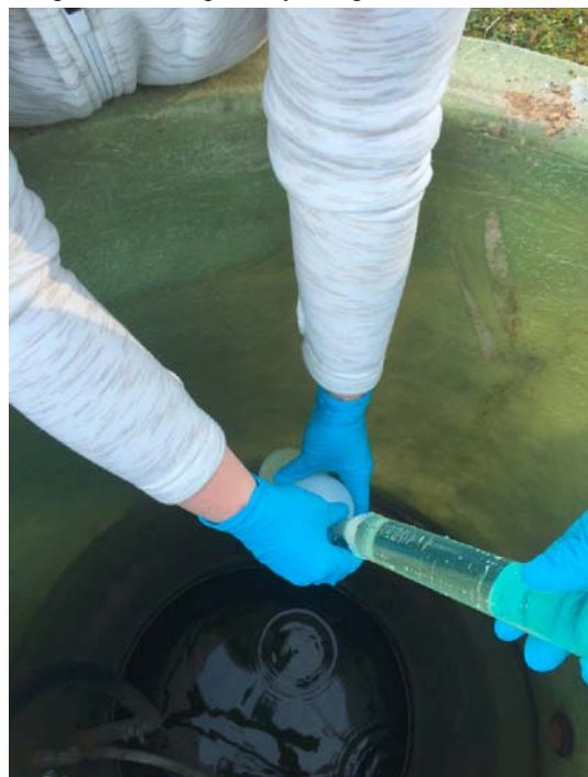
Photo No. IMG_3140; Taken on 12/09/15 at 14:02 hours by START-ET. Facing Down. TechLaw Scientists using the bailer to collect WG-SP-0003/dup WG-SP-0004.
