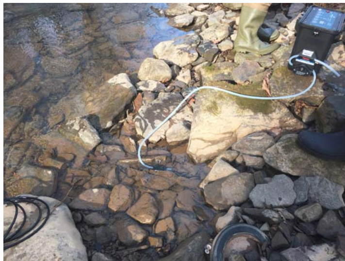
Photo No. IMG_3130; Taken on 12/09/15 at 13:08 hours by START-JW. Facing Down. The Set up used by TechLaw to collect sample WG-SW-0020
