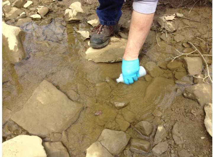
Photo No. IMG_2714; Taken on 03/24/15 at 14:23 hours by START-JW. Facing Down. START team member collecting sample WG-SW-04 by collecting surface water in a dedicated clean sample jar and purging it into the sample bottles.
