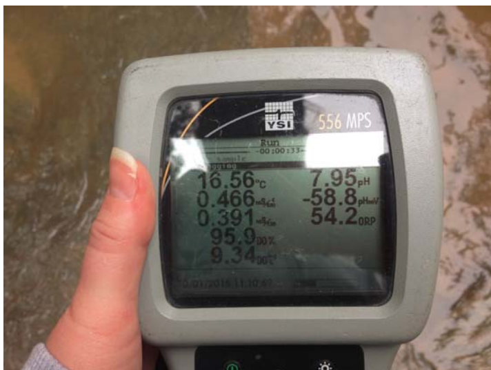
Photo No. IMG_3096; Taken on 10/01/15 at 12:15 hours by START-JW. Facing Down. Water quality measurements at sample collection location WG-SW-001, sample number WG-SW-0012/dup WG-SW-0016
