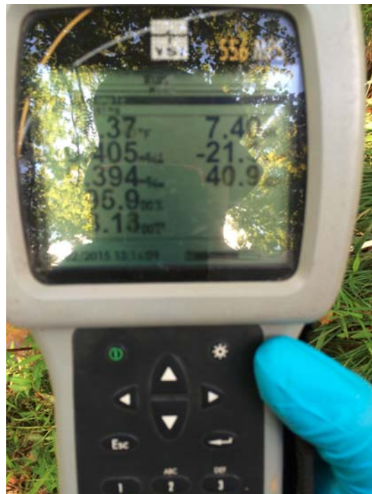
Photo No. IMG_0528; Taken on 07/22/15 at 15:27 hours by START-BH. Facing Down. YSI Meter face. Water quality measurements in stream during sampling of WG-PW-0001.
