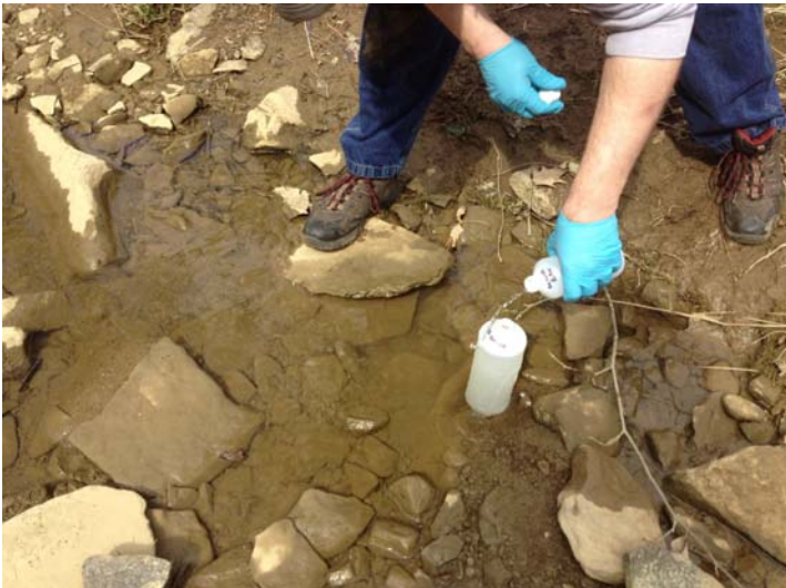
Photo No. IMG_2715; Taken on 03/24/15 at 14:26 hours by START-JW. Facing Down. START team member collecting sample WG-SW-04 by collecting surface water in a dedicated clean sample jar and purging it into the sample bottles.
