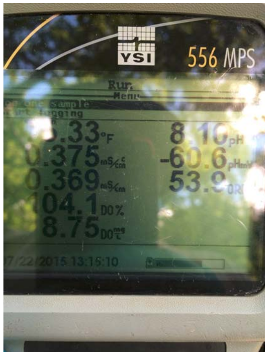
Photo No. IMG_0527; Taken on 07/22/15 at 15:26 hours by START-BH. Facing Down. YSI Meter face. Water quality measurements in stream during sampling of WG-PW-0001.
