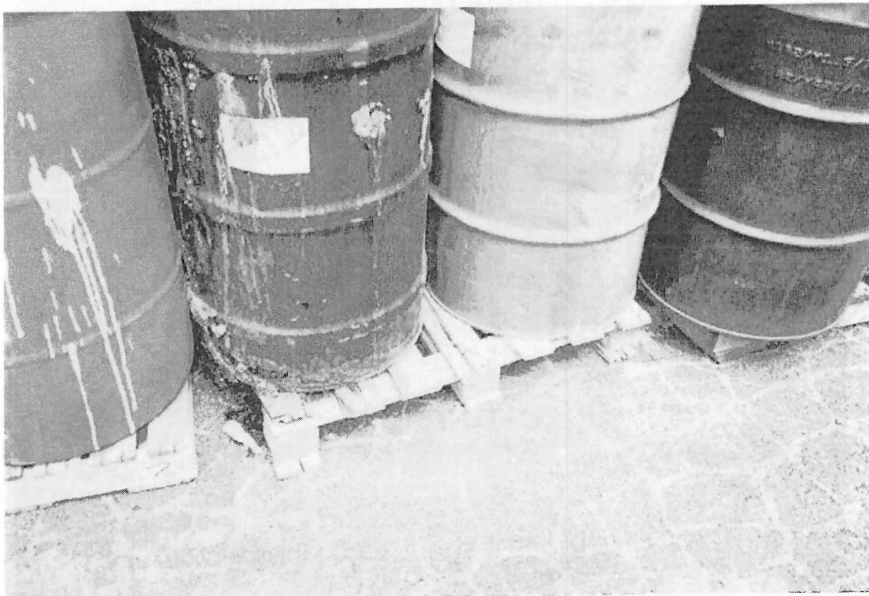
Outside Storage Area: Failing Drum Leaking Contents
