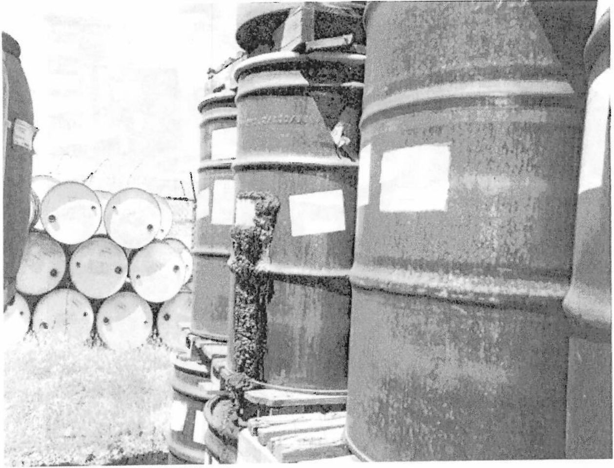
Outside Storage Area: Compromised Drum Leaking Contents
