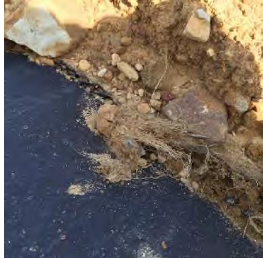
Photo 2-3: Repository cover soil consisting of an earth-rock mixture
