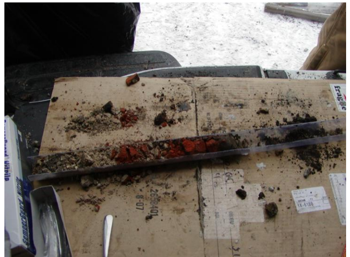
Soil Boring #9, bricks in fill
