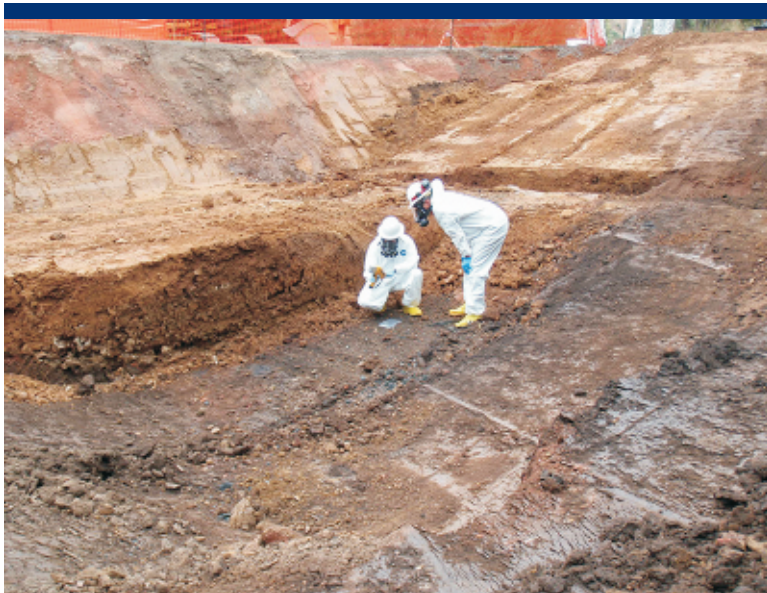
Photo 27 Field screening of soil using the XRF at the former Mill Site.
