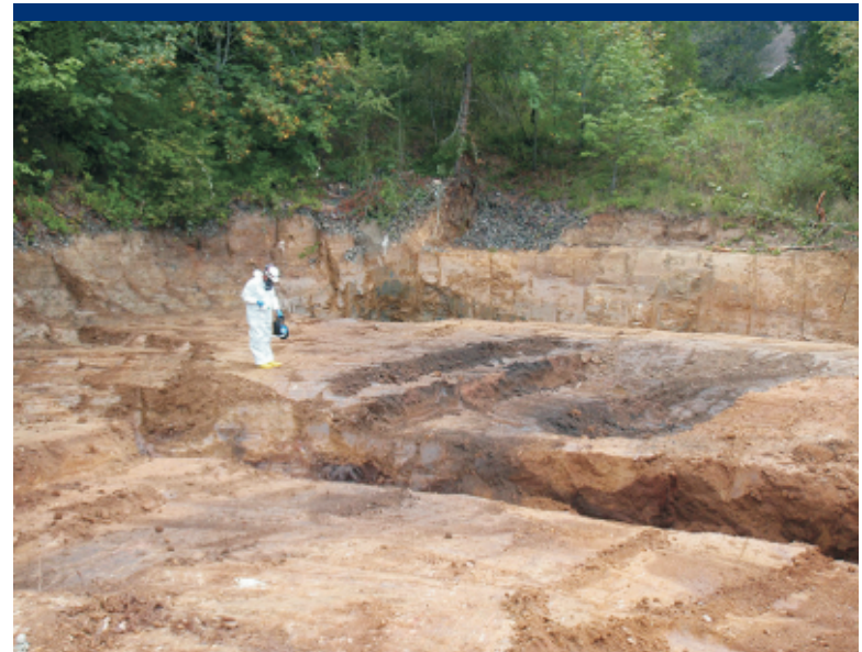
Photo 28 Field screening for mercury vapors at the former Mill Site.
