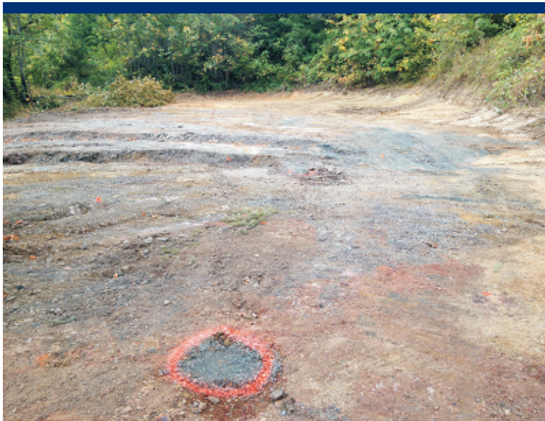
Photo 52 Two boreholes with elevated mercury vapors were filled with bentonite and marked with paint in Residence 1.
