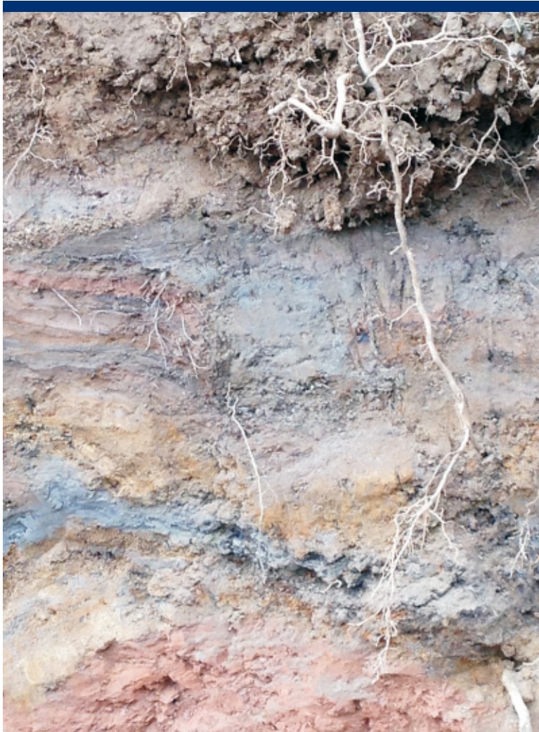
Photo 33 Sidewall in Area 2 containing visible layers of discolored soil.
