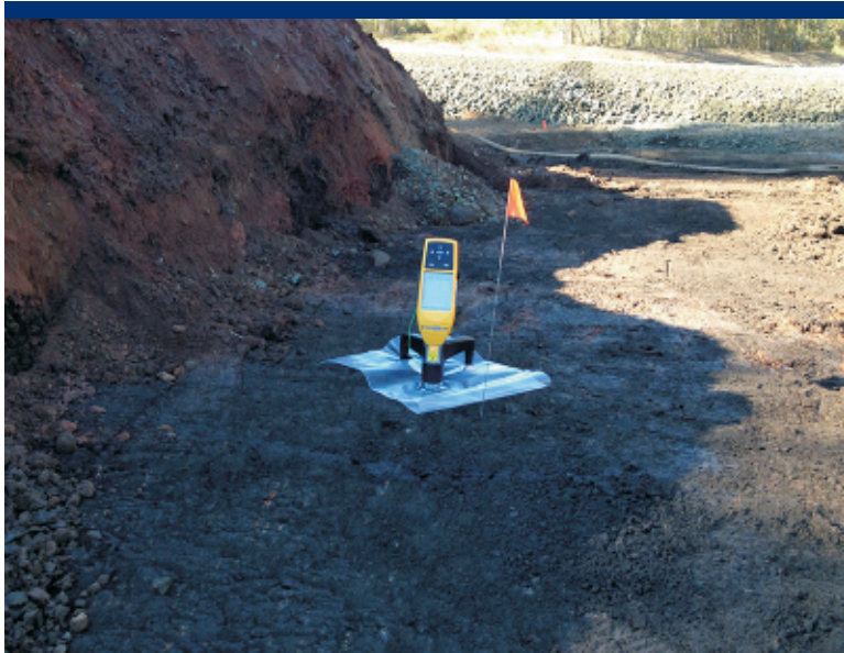
Photo 54 Field screening with the XRF in Area 1.
