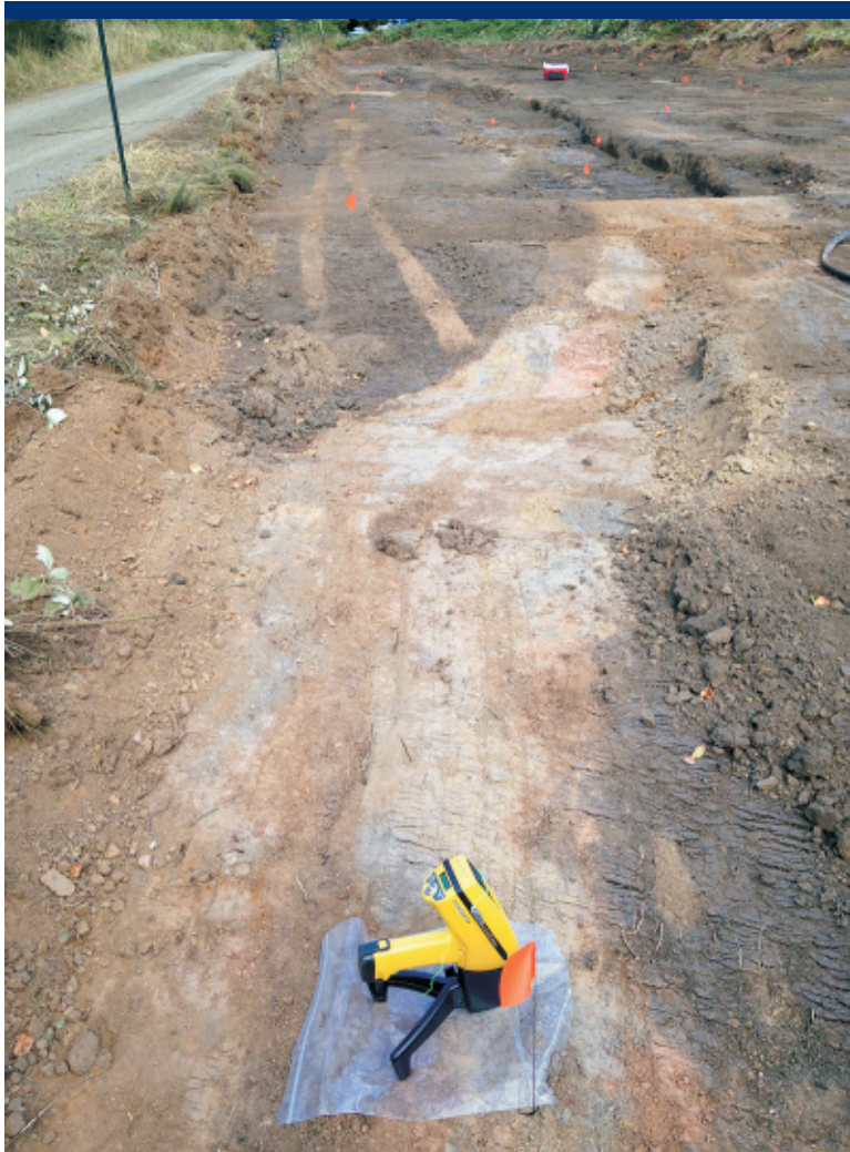
Photo 42 Field screening of discolored soil using the XRF in the southwest section of Area 4.
