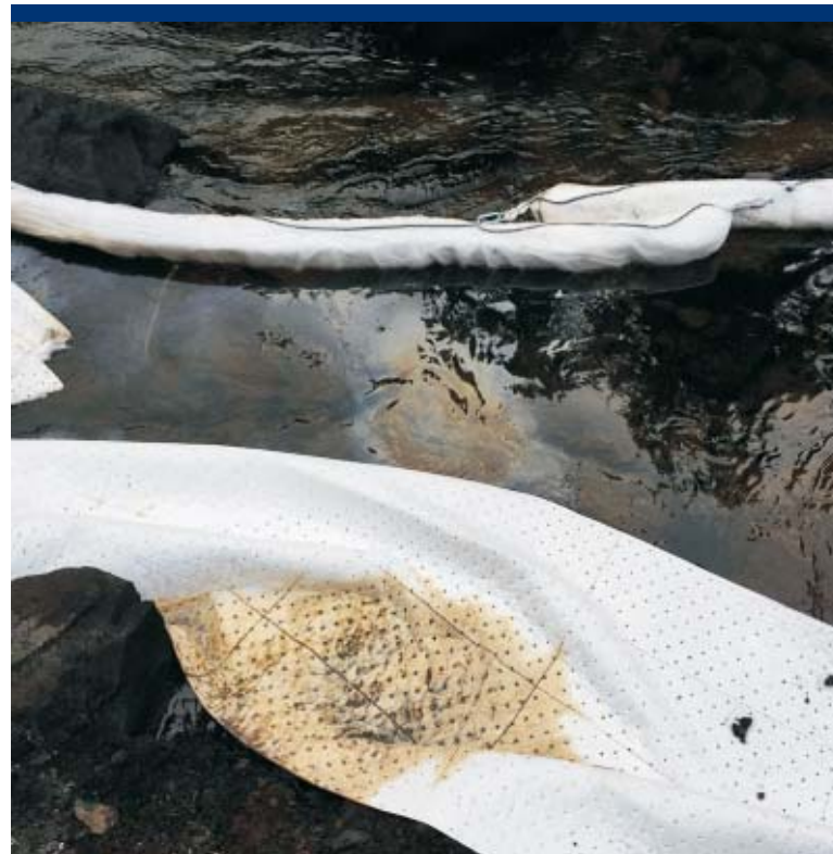
Photo 4 Air Monitoring location #9 - Inside the boom, note the sheen on the river and product adsorbed by the pads.
