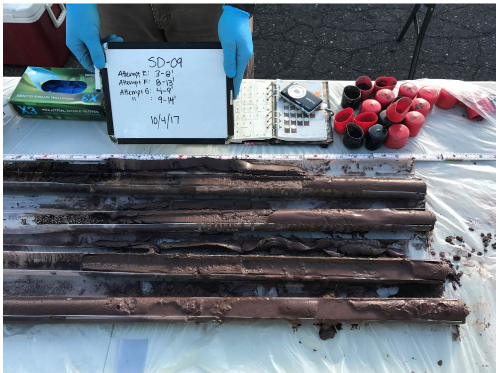
Photo 39: View of partially split bottom portions of Attempt E (3-8'; top), Attempt F (8-13'; second from top), Attempt G (4-9'; second from bottom), and Attempt G (9-14'; bottom) at SD-09
