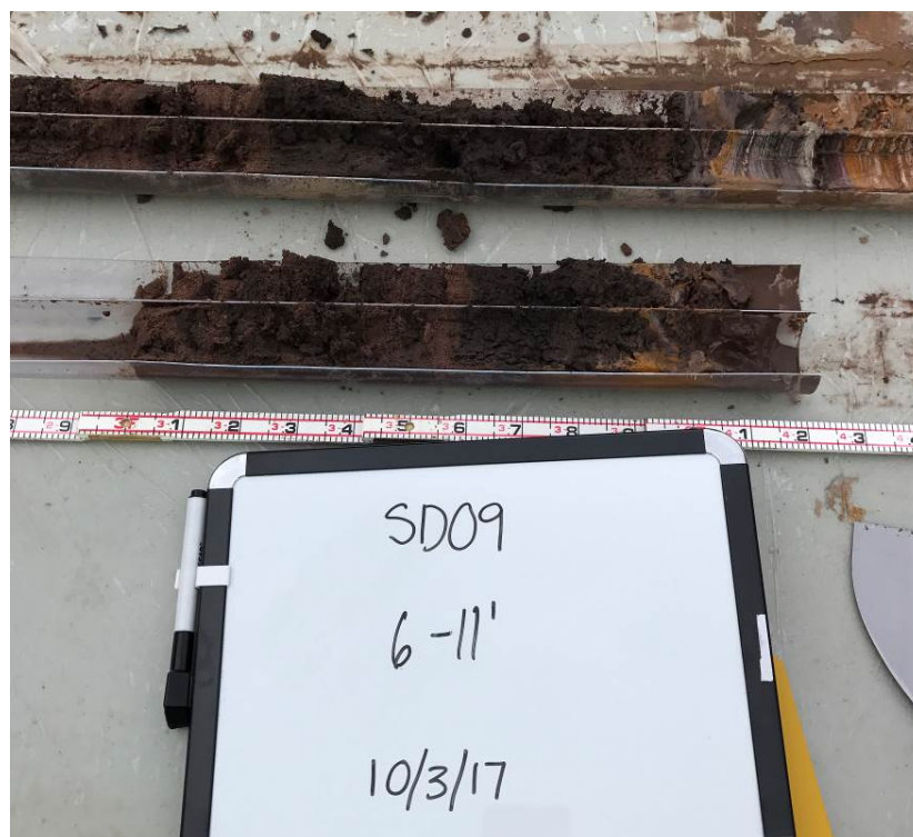
Photo 36: View of split bottom portions of Attempt B (0-6'; top) and Attempt B (6-11'; bottom) at SD-09
