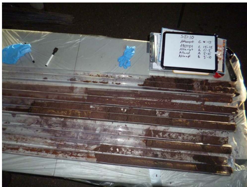
Photo 42: View of split full cores of Attempt C (8-13'; top), Attempt C (13-18'; second from top), Attempt A (0-5'; middle), Attempt A (5-10'; second from bottom), and Attempt B (5-10'; bottom) at SD-10
