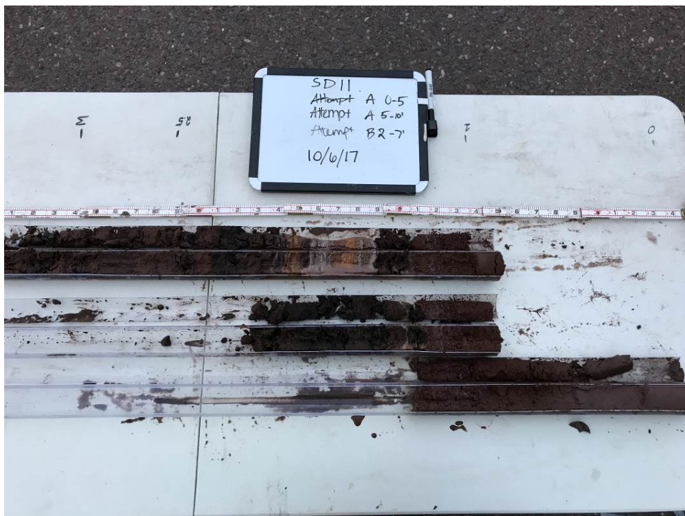
Photo 43: View of split full cores of Attempt A (0-5'; top), Attempt A (5-10'; middle), and Attempt B (2-7'; bottom) at SD-11
