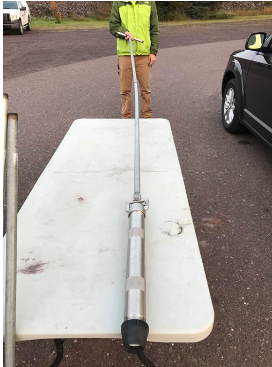
Photo 7: View of the sediment sampling apparatus with an extender pole attached
