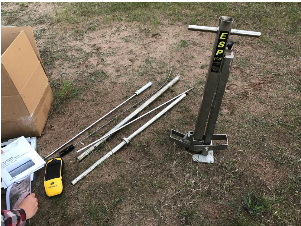
Photo 4: View of the soil sampling apparatus and GPS unit
