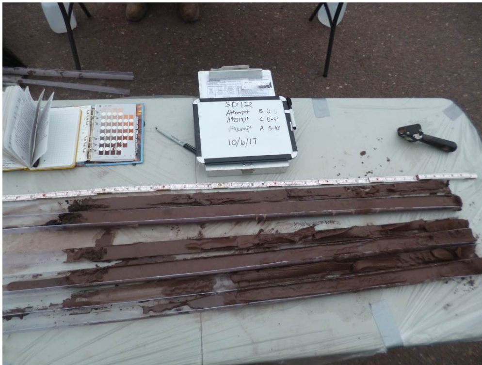
Photo 47: View of full split cores of Attempt B (0-5'; top), Attempt C (0-5'; middle), and Attempt A (5-10'; bottom) at SD-12
