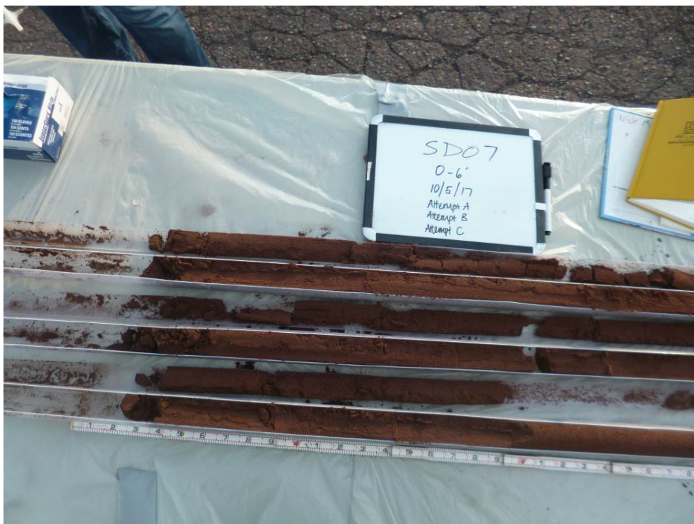
Photo 28: View of split top portions of Attempt A (top), Attempt B (middle), and Attempt C (bottom) at SD-07 (0-6' cores)
