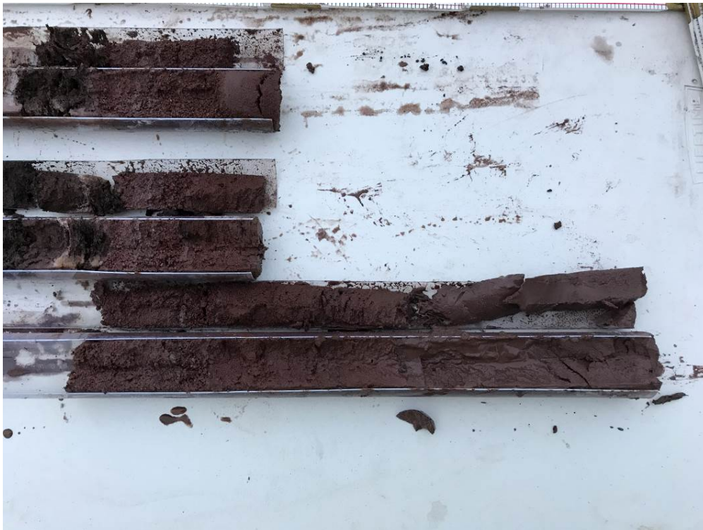
Photo 45: Close up view of very bottom portions of Attempt A (0-5'; top), Attempt A (5-10'; middle), and Attempt B (2-7'; bottom) at SD-11
