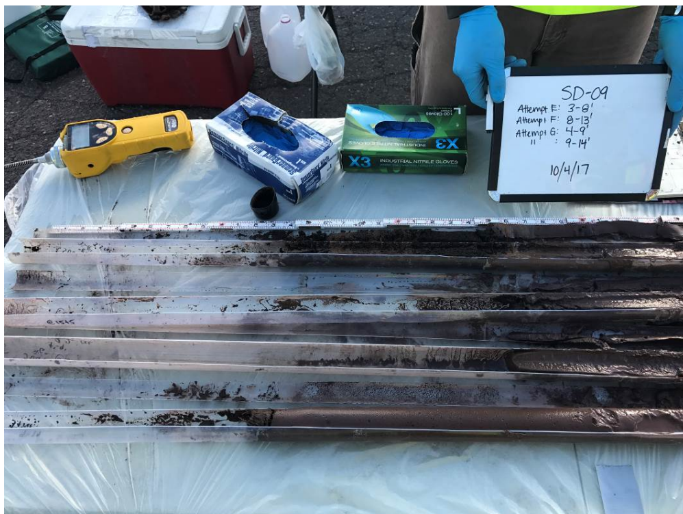
Photo 38: View of partially split top portions of Attempt E (3-8'; top), Attempt F (8-13'; second from top), Attempt G (4-9'; second from bottom), and Attempt G (9-14'; bottom) at SD-09
