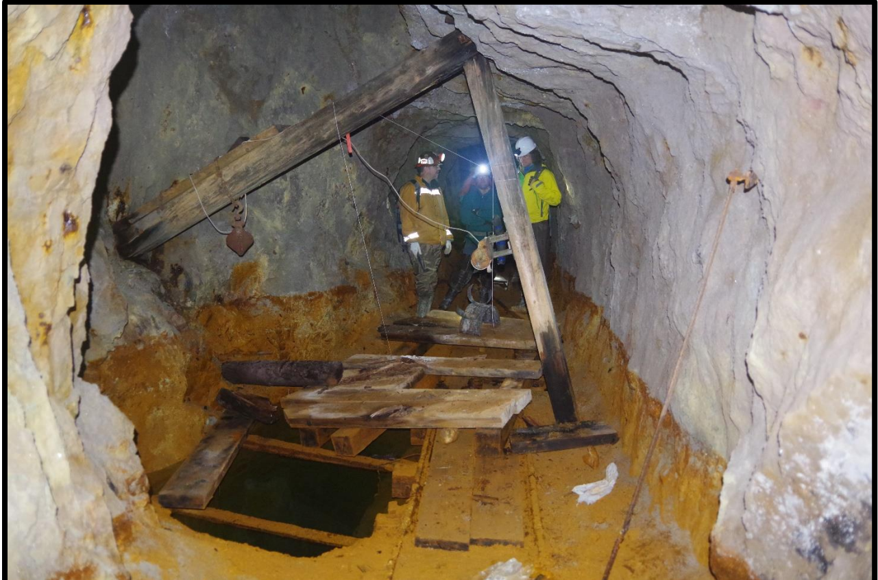
Photo 60: Del Monte Raise 53+15; Note sampling platform
