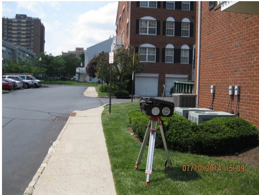
Photograph 1: On July 10, 2014, RST 3 conducted baseline particulate monitoring using DataRam 4™ particulate monitors and ambient air sampling using filter media connected to SKC air sampling pumps. From July 17, 2014 through November 14, 2014, RST 3 conducted daily particulate monitoring and air sampling during the Removal Action at the Site.
