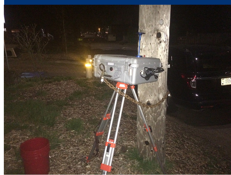
Photo 22 Secured DustTrak air monitoring station, located at NE Emerson and NE 70th Ave.
