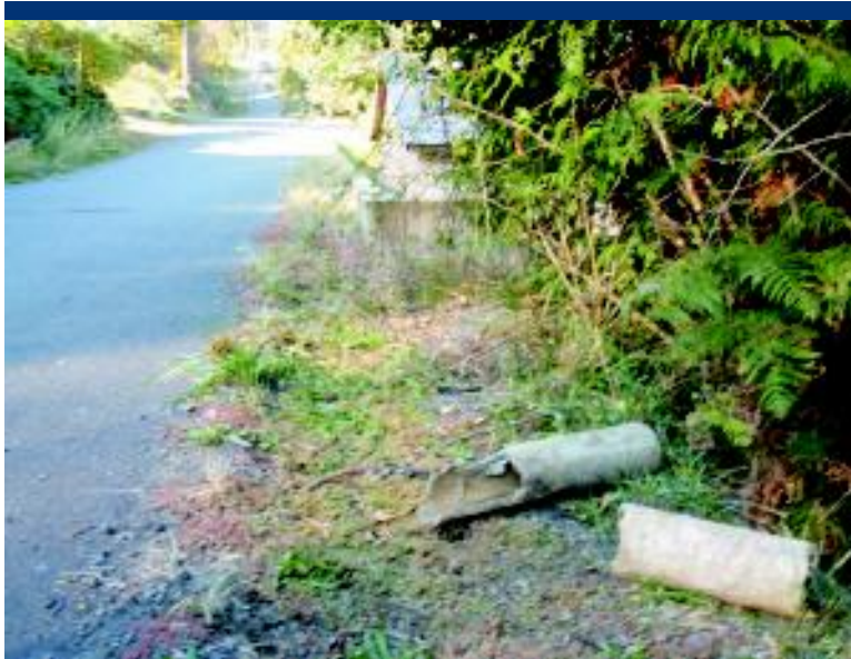
Photo 1 Asbestos-containing pipe (ACP) along Hartford Avenue (right of way).
