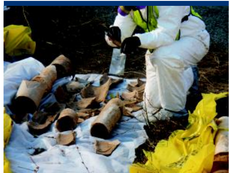
Photo 20 ERRS collects a bulk sample from recovered section of ACP.
