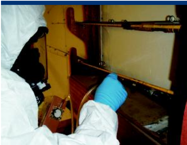
Photo 23 START collects MicroVac dust sample BK-01-MV.
