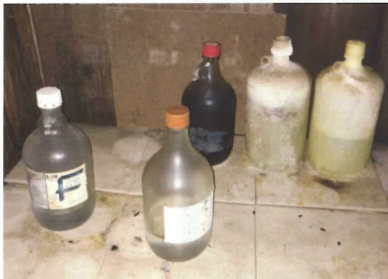
Image 8: Hi-hazard items in laboratory next to the fume hood in the lab. One is presumed Picric Acid.
