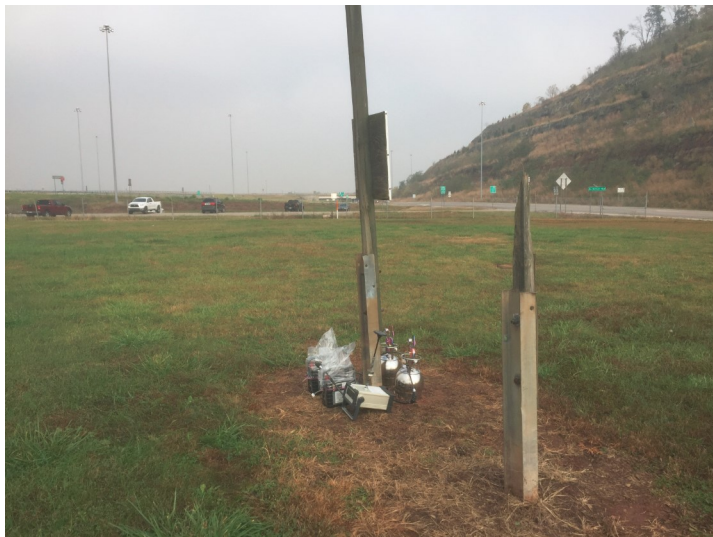
Photo No. IMG_1112; Taken on 10/26/17 at 10:48 hours by START- [REDACTED] Facing NW. Air monitoring equipment and co-located summa canister air samplers set up at the Park N' Ride monitoring location.
