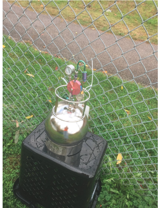
Photo No. IMG_1139; Taken on 11/02/17 at 12:21 hours by START- Air sampling with summa cannister at air sampling location at Jefferson Elementary School.
