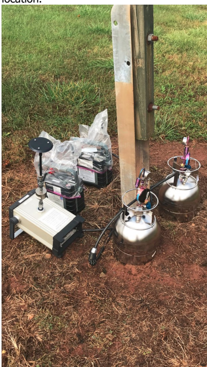
Photo No. IMG_1808; Taken on 10/26/17 at 10:47 hours by START-█ Facing N. Air monitoring equipment and summa canister air sampler set up at the Park N' Ride monitoring location.
