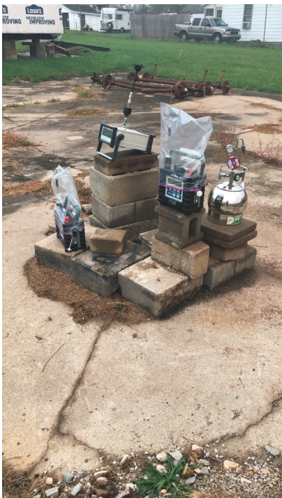
Photo No. IMG_1813; Taken on 10/26/17 at 10:28 hours by START-█ Facing N. Air monitoring equipment and summa canister air sampler set up at the Source Area Perimeter monitoring location.
