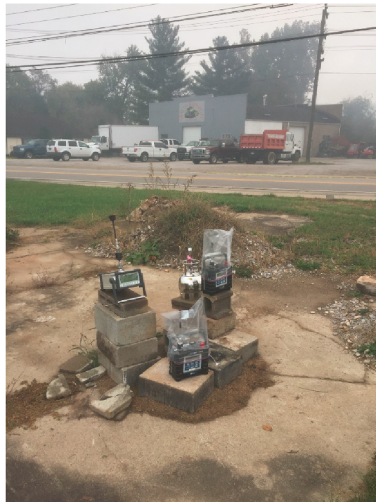
Photo No. IMG_1110; Taken on 10/26/17 at 10:29 hours by START-█ Facing N. Air monitoring equipment and summa canister air sampler set up at the Source Area Perimeter monitoring location.
