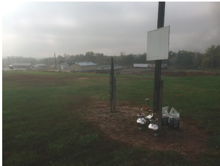
Photo No. IMG_1113; Taken on 10/26/17 at 10:48 hours by START- [REDACTED] Facing S. Air monitoring equipment and co-located summa canister air samplers set up at the Park N' Ride monitoring location. Visible smoke in background.
