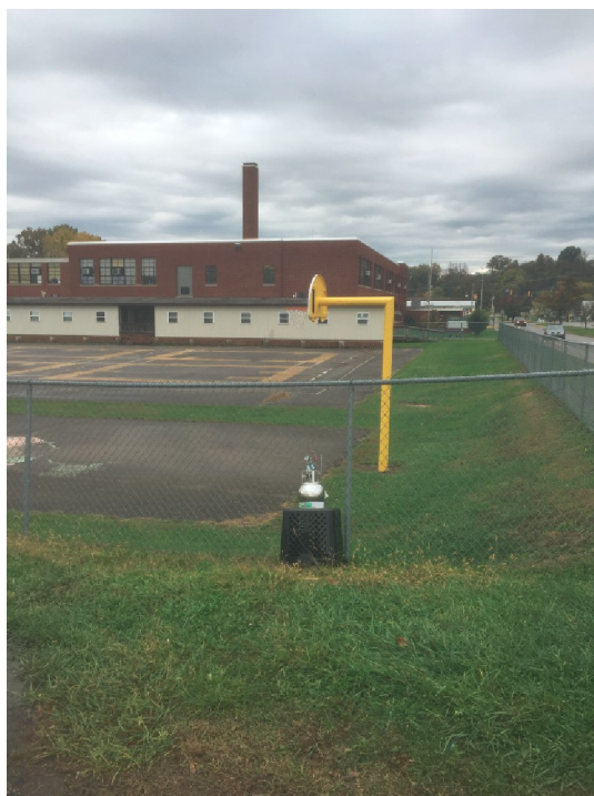
Photo No. IMG_1134; Taken on 11/02/17 at 11:48 hours by START- [REDACTED] Facing N. Air sampling with summa canister at Fairplains Elementary School during second round of air sampling.
