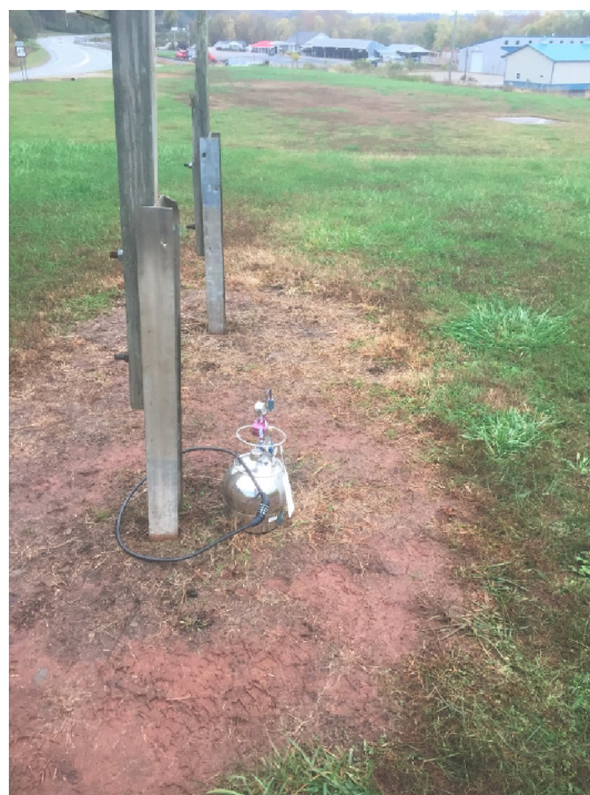
Photo No. IMG_1132; Taken on 11/02/17 at 9:09 hours by START [REDACTED] Facing SE. Air sampling with summa canister at the Park N' Ride monitoring location during second round of air sampling.
