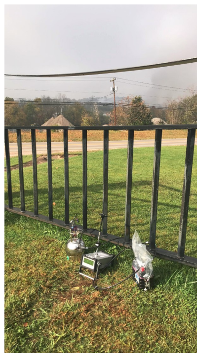
Photo No. IMG_1809; Taken on 10/26/17 at 10:53 hours by START- [REDACTED] Facing SW. Air monitoring equipment set up at the Mine Outfall/Fence monitoring location.
