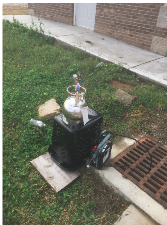
Photo No. IMG_1137; Taken on 11/02/17 at 12:12 hours by START- [REDACTED] Facing W. Air sampling with summa canister at the Rescare facility location during second round of air sampling.
