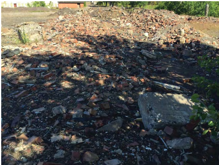
Photograph 10: WP-10 containing fire brick, much of which has a partial black coating, along with concrete, metal, and wood pieces. Photograph by J. Chrestensen, July 20, 2016.
