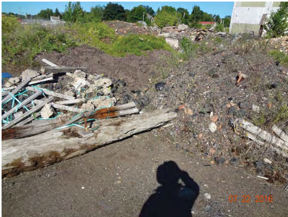
Photograph 24: WP-24 containing slag, gravel, wood, concrete, clay pipe pieces, cable, and wire. The asphalt in the background is WP-26. Photograph by MDEQ-GSU, July 22, 2016.
