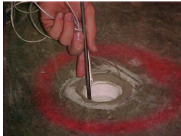
Initial insertion into permanent sampling port.
