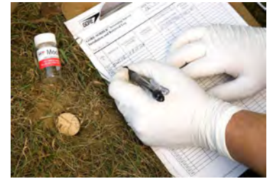
After insertion, impermeable cork sealed
