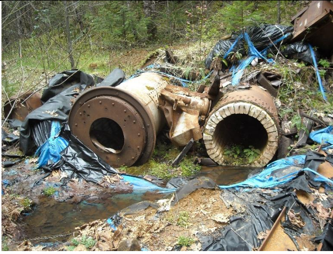
View of Brick-Lined Rotary Kiln in Scrap Repository, Note Process Residuals and Torn Visqueen
