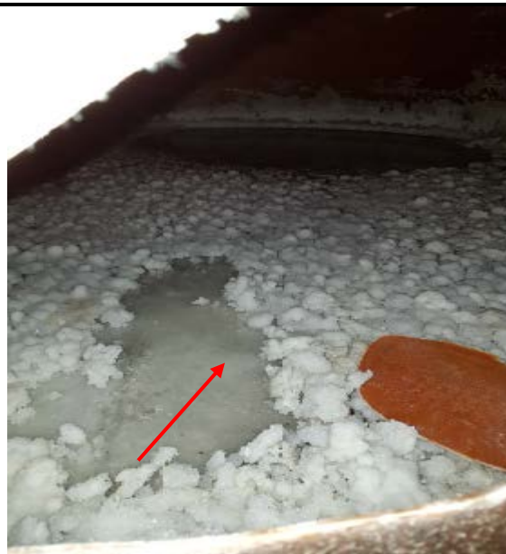
Solid ammonium hydroxide about 1 inch at bottom of tank-1 Color: White Sample ID: 2-2
