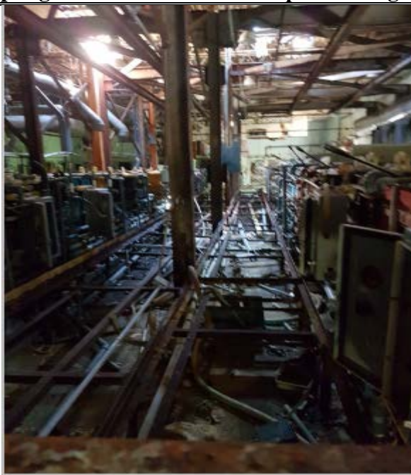
Two lines of plating bath. Each line contain 15 rectangular bath tank.
