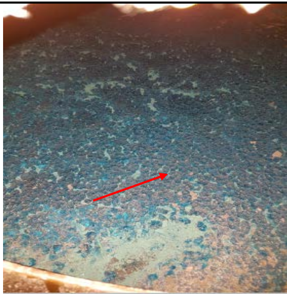
Solid ammonium hydroxide about 1 inch at bottom of tank-1 Color: blue Sample ID: 2-1
