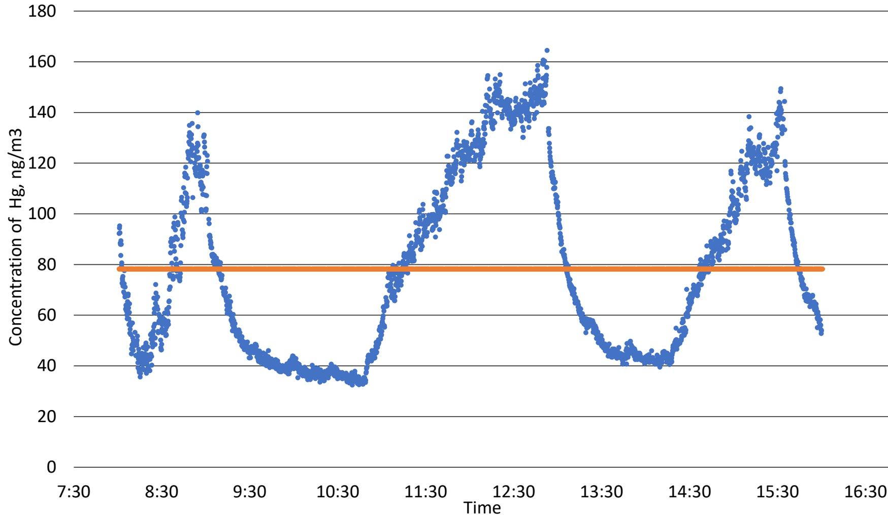
CDPHE Mercury Spill clearance run with the Lumex mercury vapor analyzer. Run completed on June 6, 2019, start time 0800, end time 1600. Average 8 hour concentration is 78ng/m<sup>3</sup> (orange line), well below established action level of 1000ng/m<sup>3</sup>. Readings conducted in spill area after EPA conducted removal actions. Readings conducted at breathing zone.
