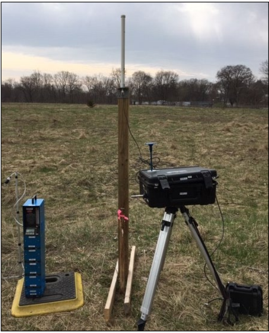
Air monitors were set out around the building to monitor for dust and asbestos fibers.
