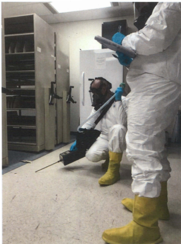
Figure 1. (Above) EPA START contractor performing storage room assessment and readings for mercury vapors utilizing Jerome (mg/m 3 ) and Lumex (ng/m 3 ) instrumentation.
