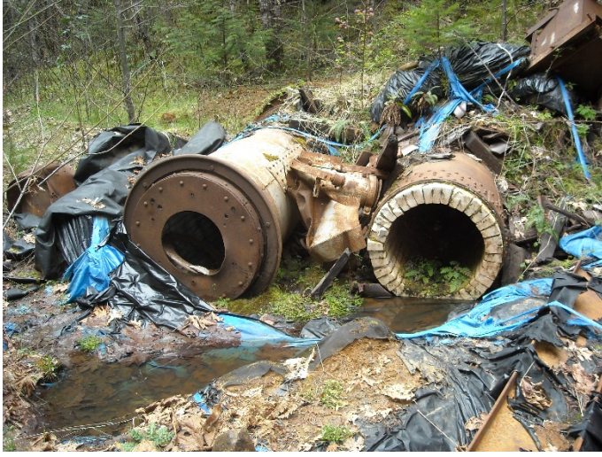
View of Brick-Lined Rotary Kiln in Scrap Repository, Note Process Residuals and Torn Visqueen
