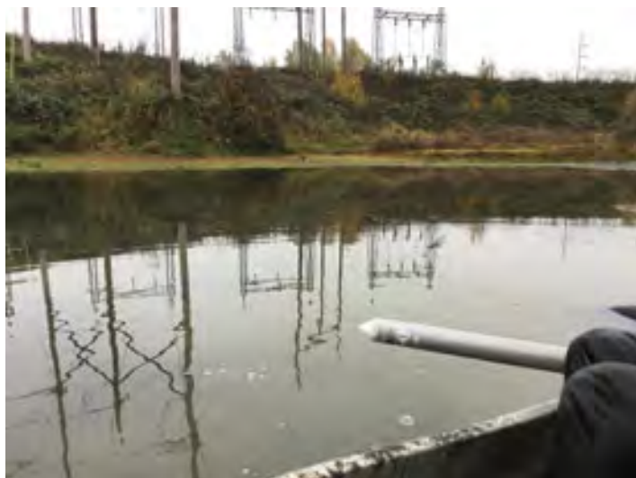
Sample borer at location SR08SD, water depth = 2'.
