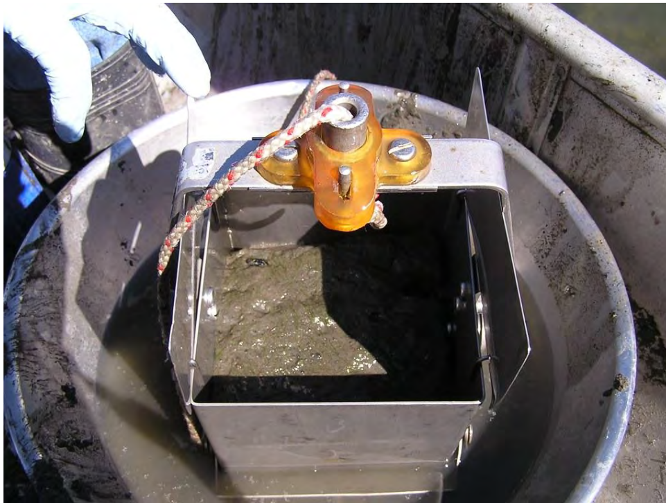
Figure 8 Ekman Dredge Sampler
