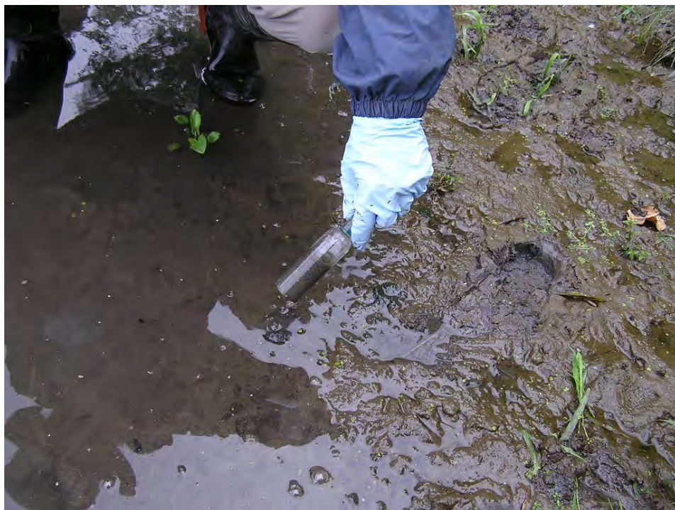
Figure 9 Glass Scoop Sediment Sampler
