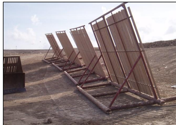
Best Practice: Portable litter fencing can be moved daily to the working face and positioned in the prevailing wind direction.
