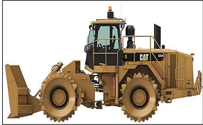
Best Practice: Landfill compactor designed to spread and compact waste.
