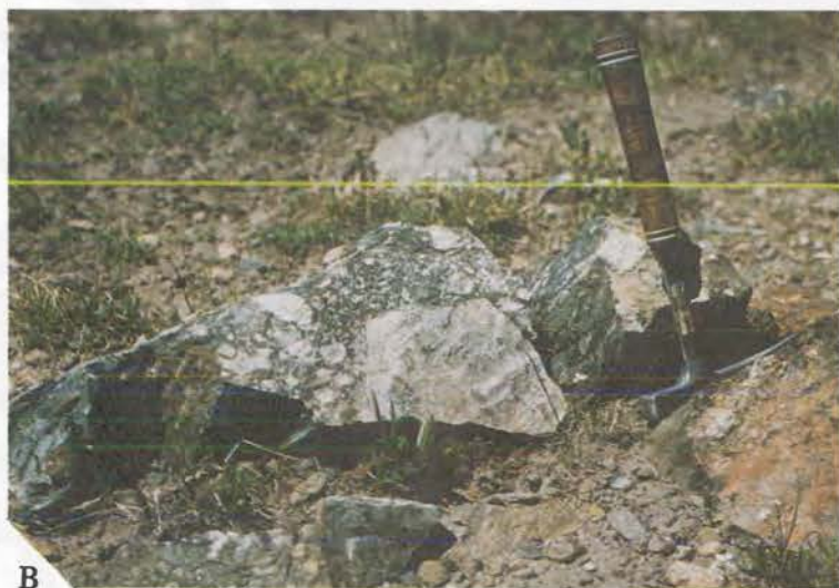
Figure 8. [Above] (A) Massive pyritized ore with colloform texture. This sample, collected in the Sierra Madre, exhibits rounded grains of pyrite mantled by chalcopyrite. The matrix is magnetite with minor chlorite. (B) "Mill rock." Felsic volcaniclastics are often found in close proximity to massive ore, as at this locality in the Sierra Madre. Felsic volcanic breccias are mapped in Canada as tracers to ore. Sangster (1973) dubbed it "mill rock" because whenever he was standing on a volcaniclastic with large fragments, he could "hear the sound of a mill." Presumably, the volcaniclastics occur near minable ore and represent a fossil volcanic orifice from which the metallic sulfides originated. Photographs by W.D.H., 1978.
