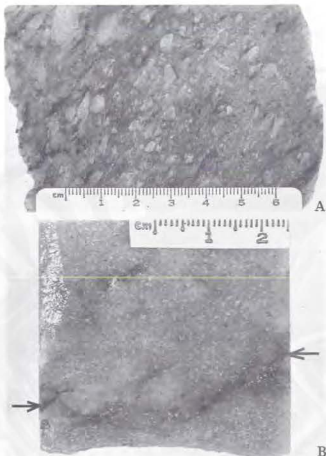
Figure 6. A and B, core splits of quartz-pebble conglomerates, Medicine Bow Mountains. (A) Grain size fining upward (top to right), typical of the metaconglomerate sequences. (B) Minor pyrite mineralization (between arrows) in weakly radioactive zone near large quartz pebbles. (C) Stretched-pebble paraconglomerate in the central Laramie Range. These types of deposits represent placer deposition in a fluvial environment. Reducing (oxygen-deficient) atmospheric conditions provided by the primitive Precambrian atmosphere were necessary to the transportation and deposition of uraninite and pyrite in the placer environment. Photographs by A.J. Ver Ploeg, 1982, W.D.H., 1980.
