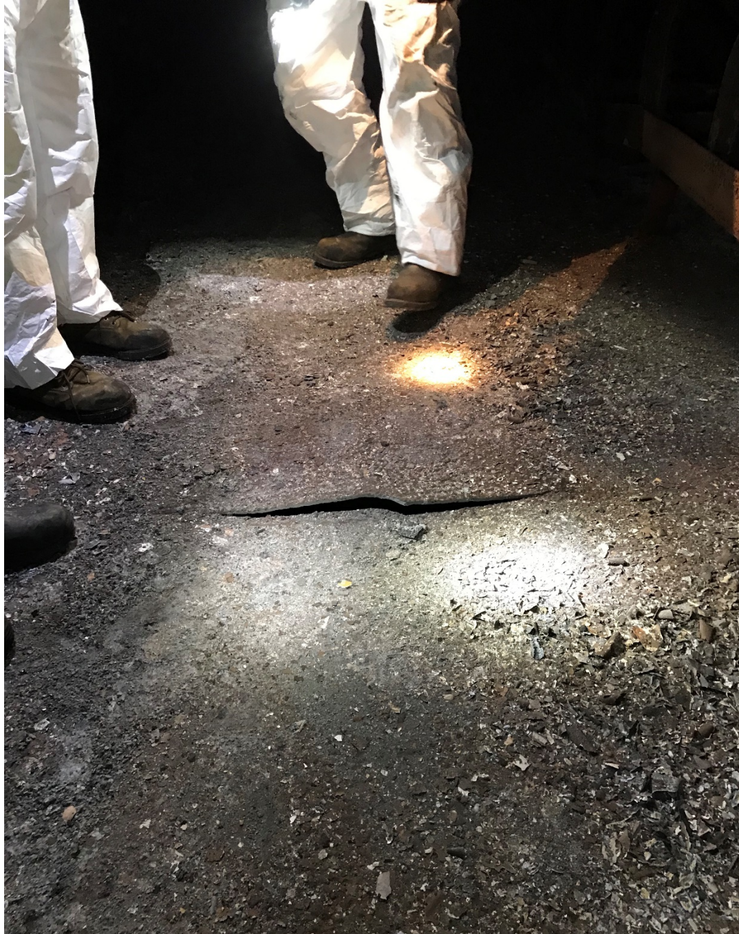
Starboard Conveyor Tunnel Deck Fracture - amidship
