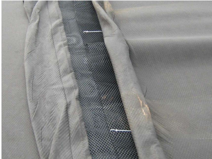
Figure 26: Geocomposite with Geonet and Geotextile
