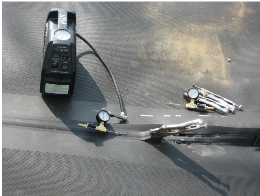
Figure 18: Air Pressure Testing of Track Welded Seam
