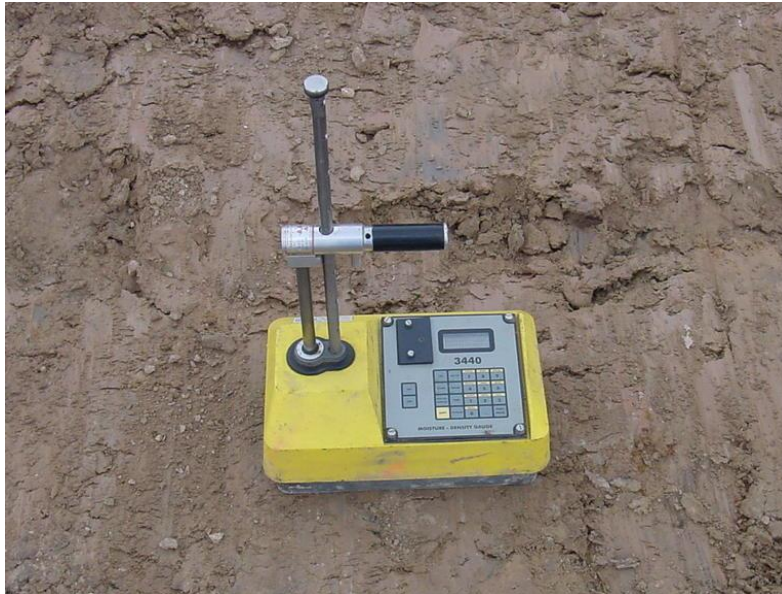
Figure 11: Nuclear Density Gage
