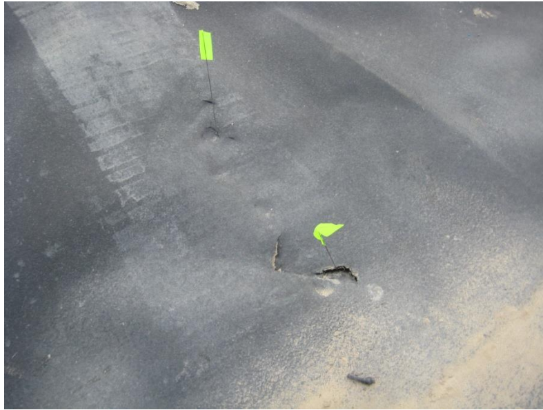
Figure 21: Damage to HDPE Liner Flagged for Repair
