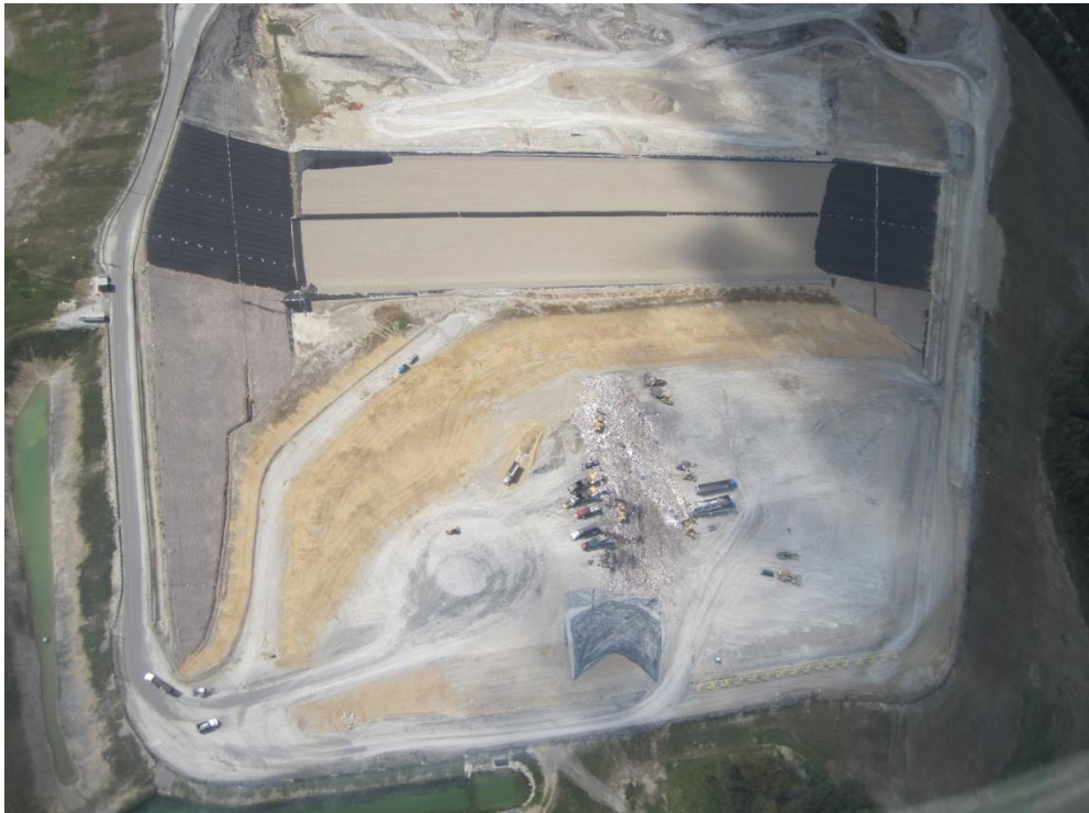
Figure 1: Aerial View of Sanitary Landfill with New Composite Liner Construction
