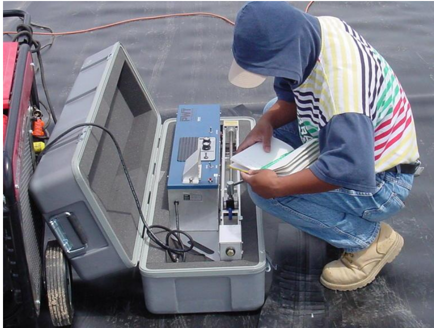
Figure 20: Destructive Testing
