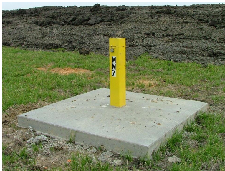
Figure 40: Groundwater Monitoring Well Completion with Casing, Lock and Concrete Pad
