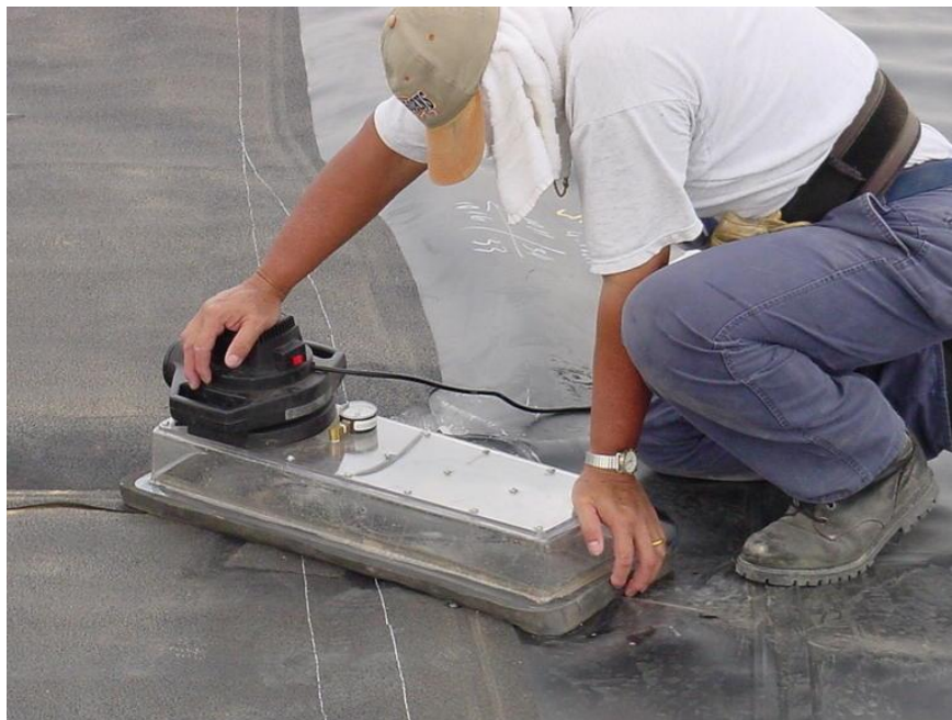
Figure 19: Vacuum Box Testing
