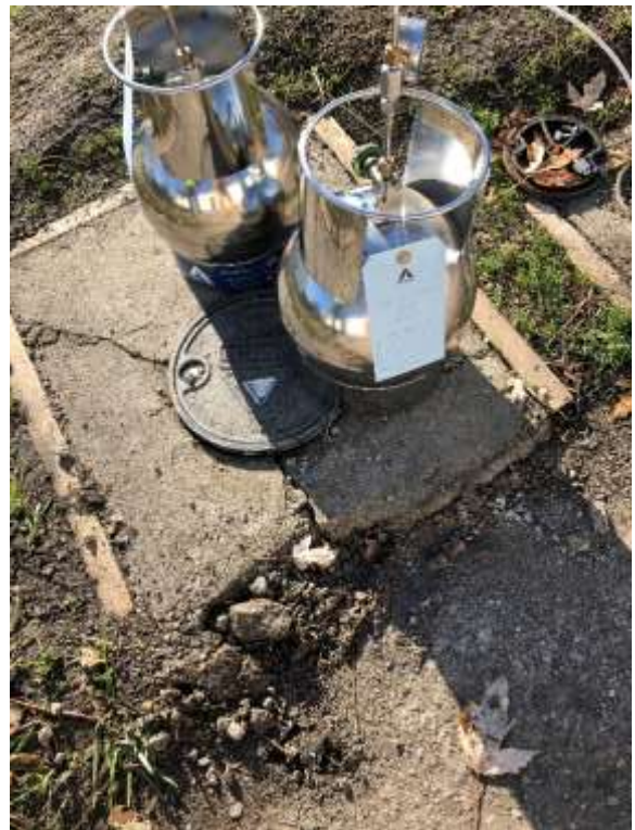
Collecting soil gas samples from monitoring wells that were installed in the fall.
