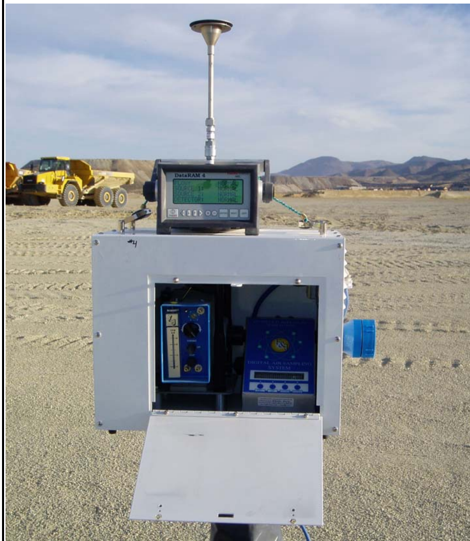
PHOTOGRAPH 21.: Air monitoring station with DataRAM 4 particulate sampler above and F&J high volume sampler below.
