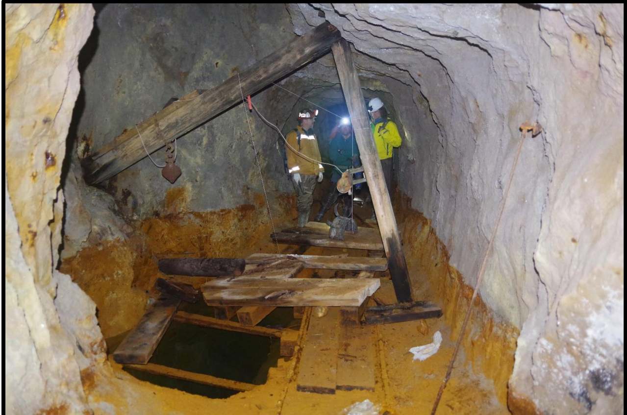
Photo 60: Del Monte Raise 53+15; Note sampling platform
