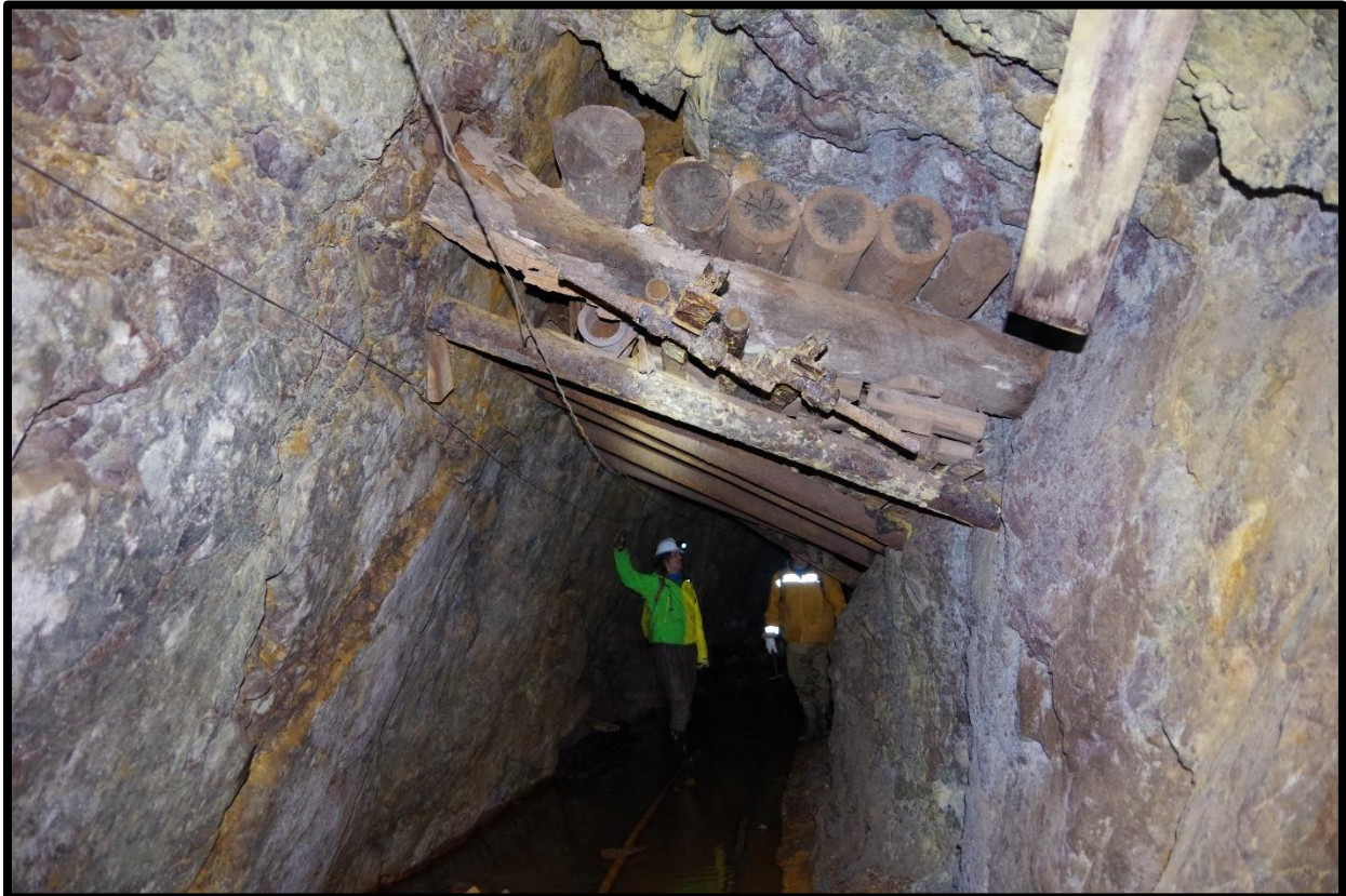
Photo 39: Steel pipe stulls near 32+20; Note pipe cribbing
