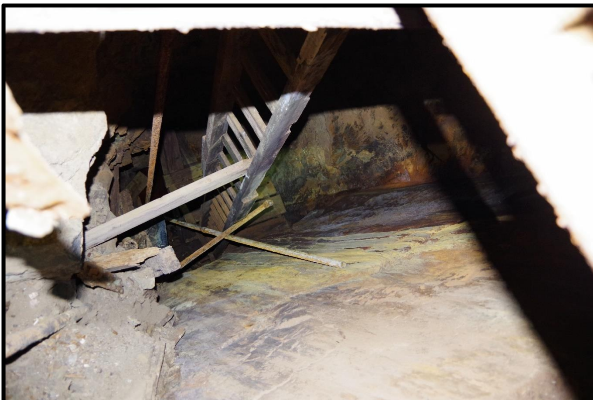
Photo 18: Looking down Daylight Winze: Note smooth footwall, ladder, and landing
