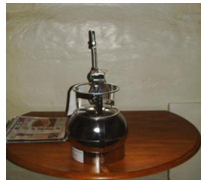
Canister Placed on Table to Collect Indoor Air Sample
