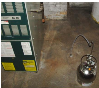
SUMMA Canister Installed in Basement
