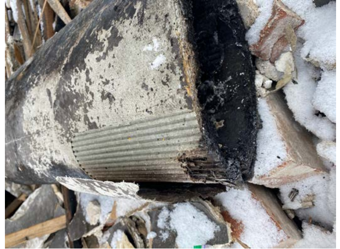
PHOTO 2- Thermal System Insulation "Aircell" debris contains asbestos
