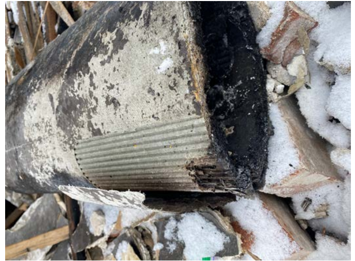
PHOTO 2- Thermal System Insulation "Aircell" debris contains asbestos
