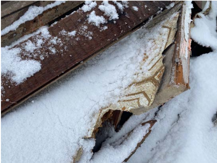
PHOTO 3- Rolled vinyl flooring debris contains asbestos
