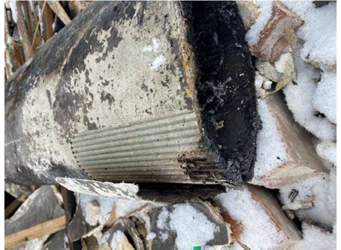
PHOTO 2- Thermal System Insulation "Aircell" debris contains asbestos
