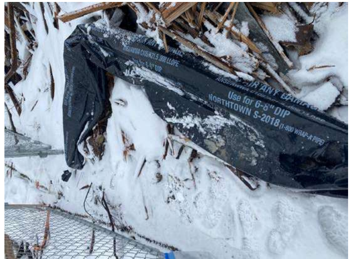
PHOTO 4- Thermal System Insulation "Aircell" debris contains asbestos (wrapped in plastic sheeting)
