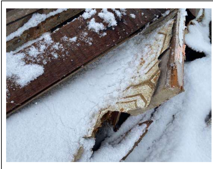
PHOTO 3- Rolled vinyl flooring debris contains asbestos
