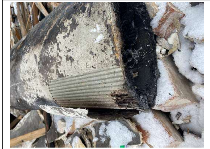
PHOTO 2- Thermal System Insulation "Aircell" debris contains asbestos
