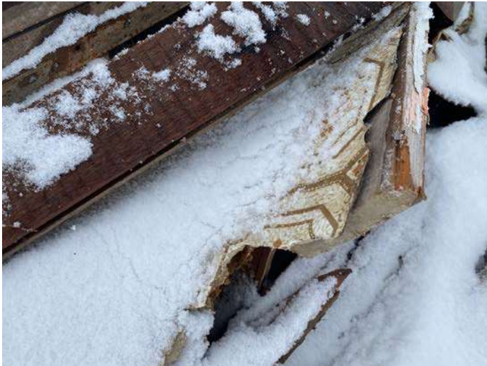
PHOTO 3- Rolled vinyl flooring debris contains asbestos
