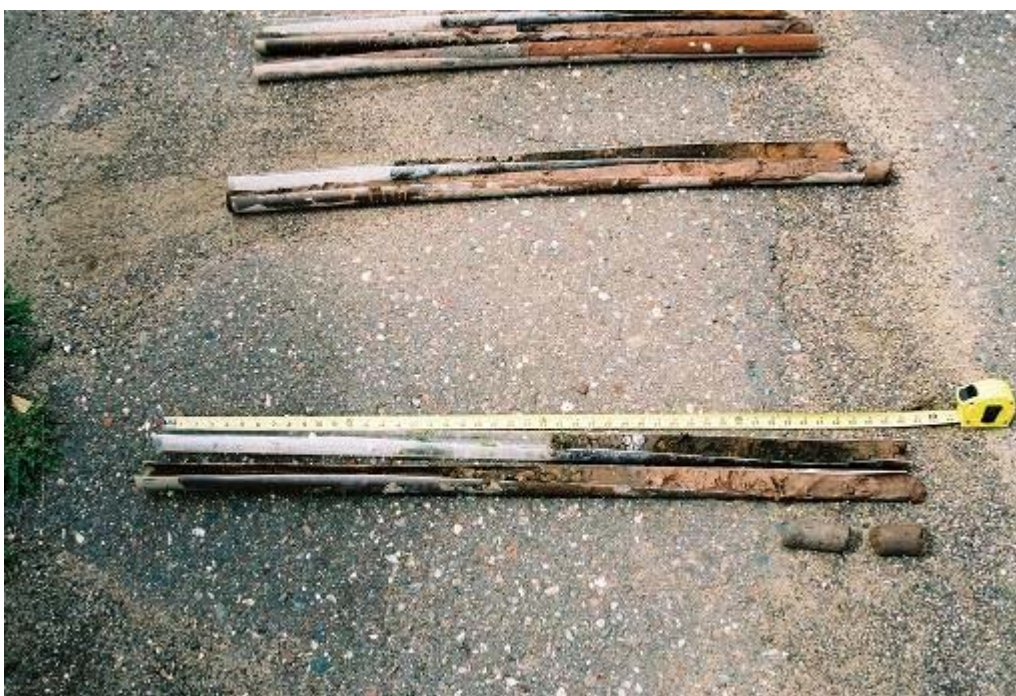
Photograph 11: 5/17/06 15:50 Soil cores at bottom of photograph from WGP-03. Shallower soils are at the top left, the bottom of the boring is at the bottom right. Photo by J. Chrestensen
