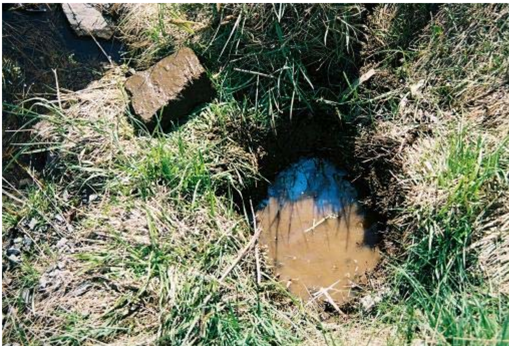
Photograph 12: 5/17/06 16:30 Sheen on groundwater in test hole approximately 10 feet west of WSS-01. Ditch stream flow approximately one foot south (left) of the test hole. Photo by J. Chrestensen
