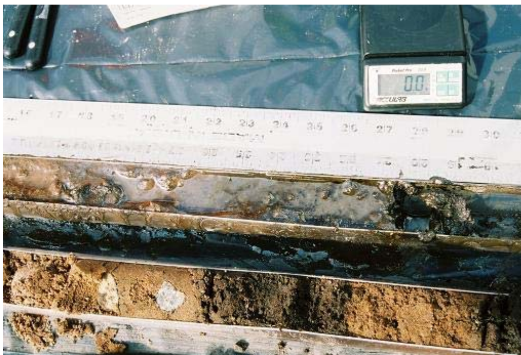
Photograph 36: 5/18/06 10:40 Detail of 6 to 7 foot interval in soil core from WGP-21. Note the visible free product. Photo by J. Chrestensen
