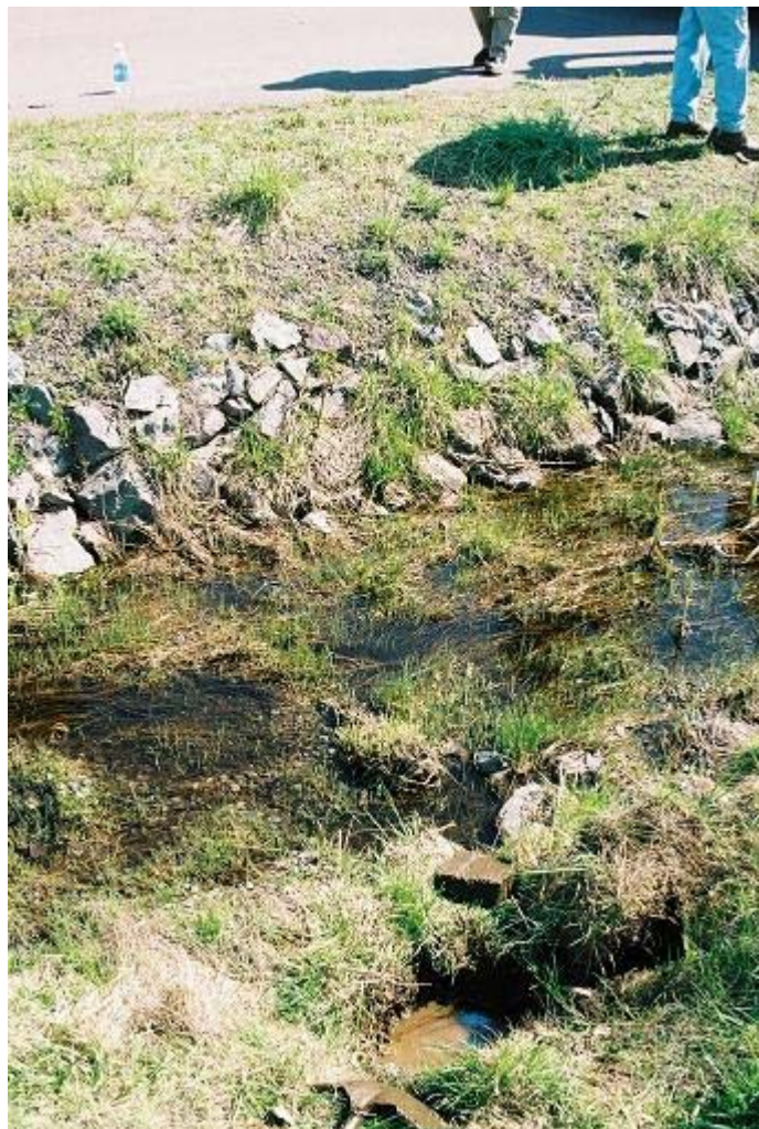
Photograph 13: 5/17/06 16:30 Looking southerly at ditch and Franklin Street from test hole approximately 10 feet west of WSS-01 location. Sheen is evident on water in the hole. Ditch stream flow approximately one foot south of the test hole. Photo by J. Chrestensen
