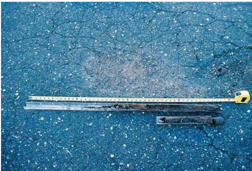
Photograph 18: 5/17/06 18:10 Soil cores from WGP-05. Shallower soils are at the top left, the bottom of the boring is at the bottom right. Photo by J. Chrestensen
