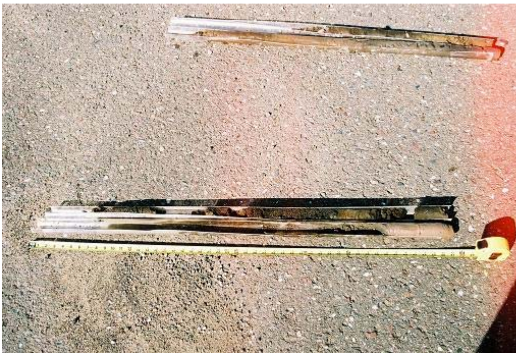
Photograph 21: 5/17/06 18:10 Soil cores at bottom of photograph from WGP-08. Shallower soils are at the top left, the bottom of the boring is at the bottom right. Photo by J. Chrestensen
