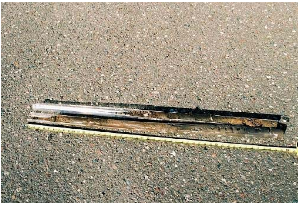
Photograph 20: 5/17/06 18:10 Soil cores from WGP-07. Shallower soils are at the top left, the bottom of the boring is at the bottom right. Photo by J. Chrestensen
