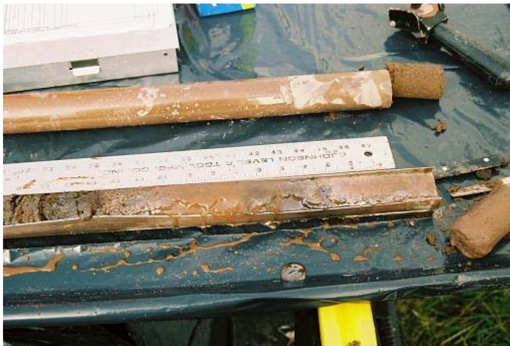
Photograph 30: 5/18/06 09:12 Detail of 6.5 to 7.5 foot interval from WGP-16. Note the sheen in the interval where dark brown free product was observed in Photograph 29 above. Photo by J. Chrestensen
