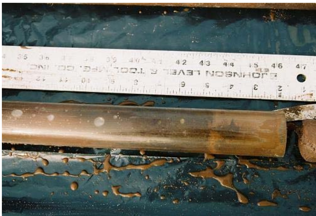
Photograph 29: 5/18/06 09:10 Detail of 6.5 to 7.5 foot interval from WGP-16. Note the dark brown free product at approximately 7 feet. Photo by J. Chrestensen
