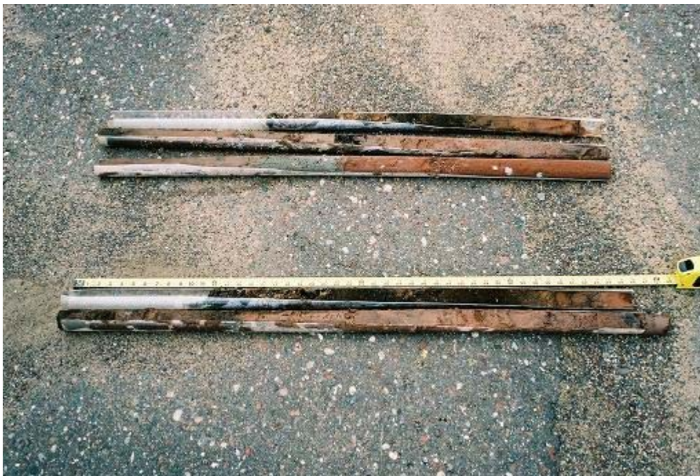
Photograph 10: 5/17/06 15:30 Soil cores at bottom of photograph from WGP-02. Shallower soils are at the top left, the bottom of the boring is at the bottom right. Photo by J. Chrestensen
