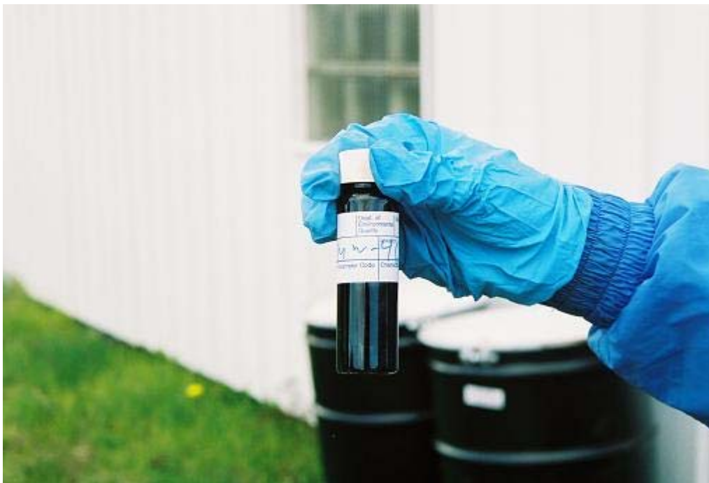
Photograph 17: 5/17/06 17:05 Vial collected by MDEQ from MW-46 on 10/12/05. Black substance on the inside surface of the vial did not move upon shaking, but there was liquid movement in the center of the vial. Photo by J. Chrestensen
