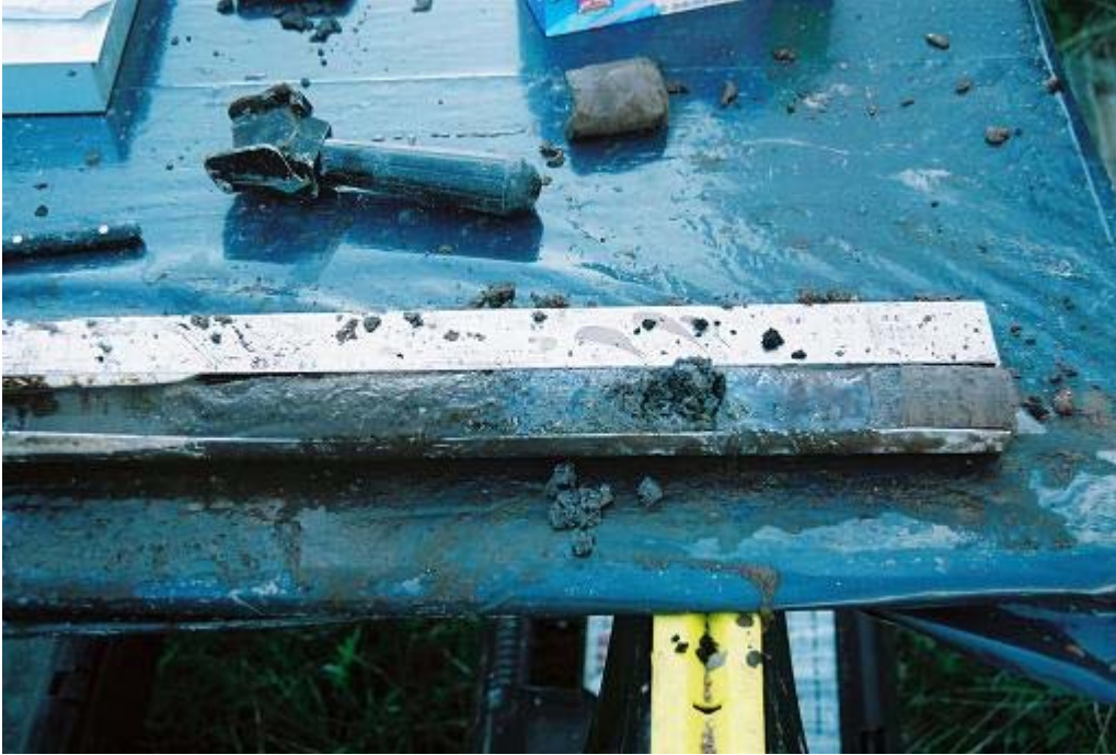
Photograph 23: 5/17/06 18:30 Detail of 6 to 7.5 foot interval in soil core from WGP-10. Note the sheen from 6.5 to 7 feet. Photo by J. Chrestensen
