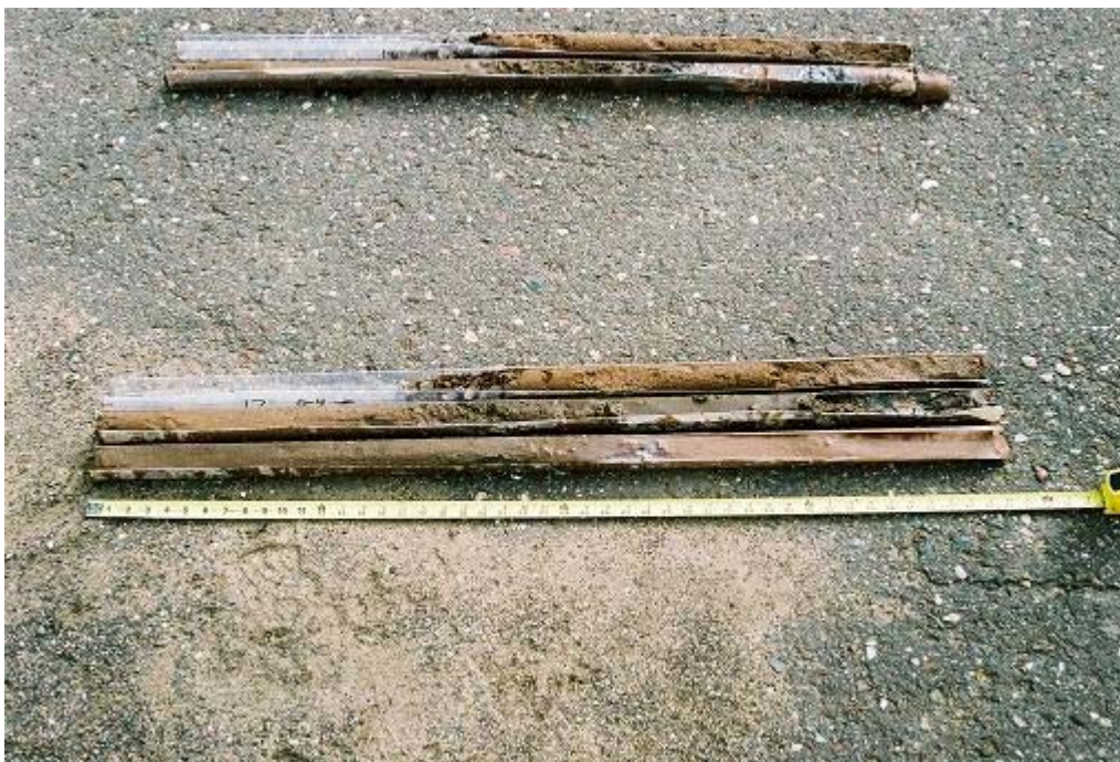
Photograph 32: 5/18/06 09:30 Soil cores at bottom of photograph from WGP-17. Shallower soils are on the left, the bottom of the boring is at the bottom right. Photo by J. Chrestensen
