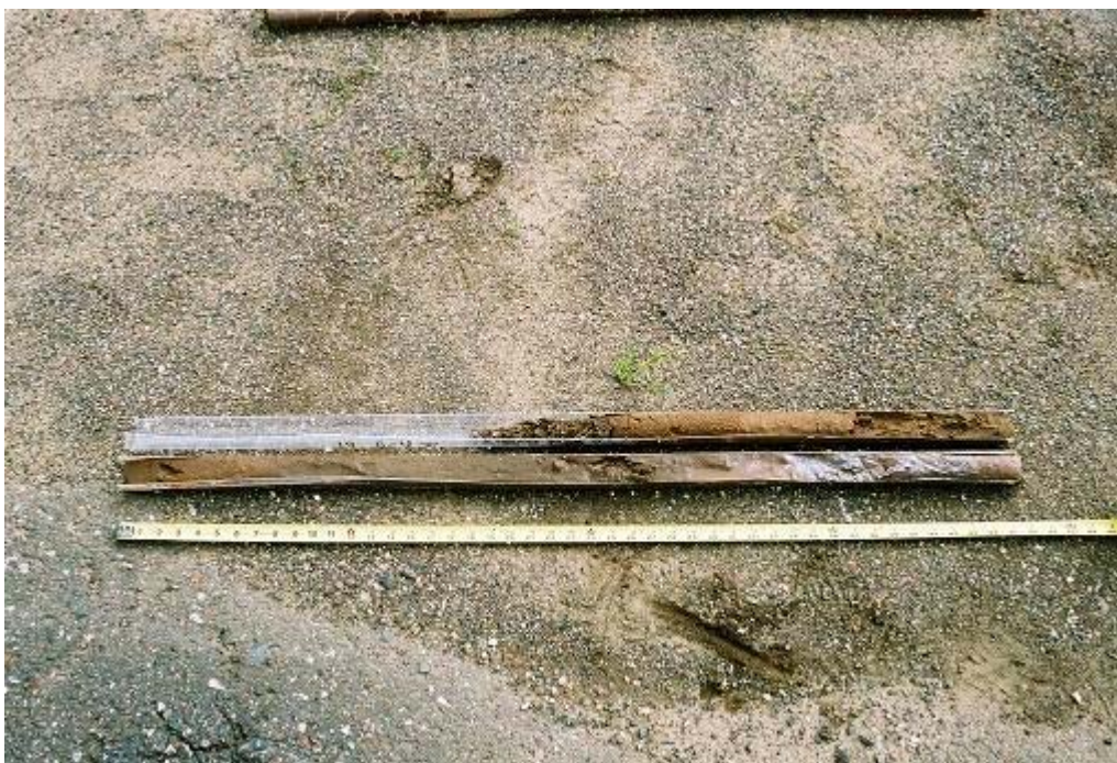
Photograph 34: 5/18/06 10:10 Soil cores from WGP-19. Shallower soils are on the left, the bottom of the boring is at the bottom right. Photo by J. Chrestensen
