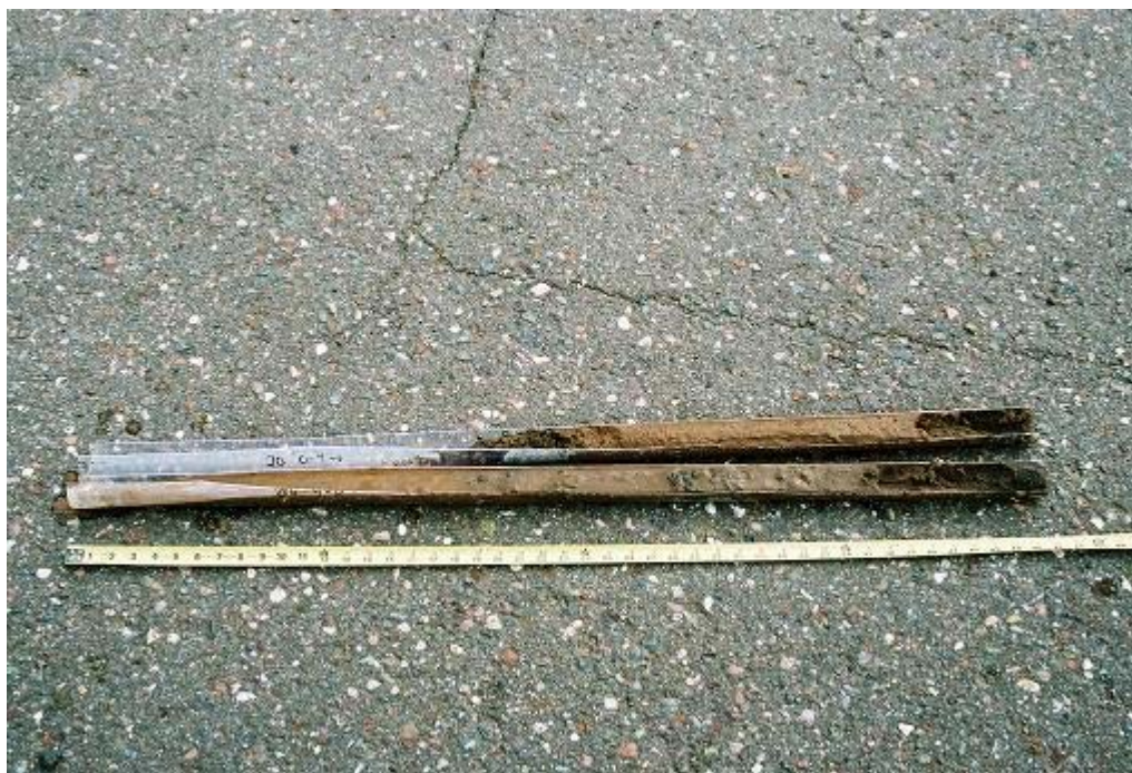
Photograph 35: 5/18/06 10:10 Soil cores from WGP-20. Shallower soils are on the left, the bottom of the boring is at the bottom right. Photo by J. Chrestensen
