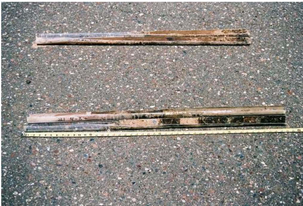
Photograph 39: 5/18/06 15:04 Soil cores at bottom of photograph from WGP-21. Shallower soils are on the left, the bottom of the boring is at the bottom right. Photo by J. Chrestensen
