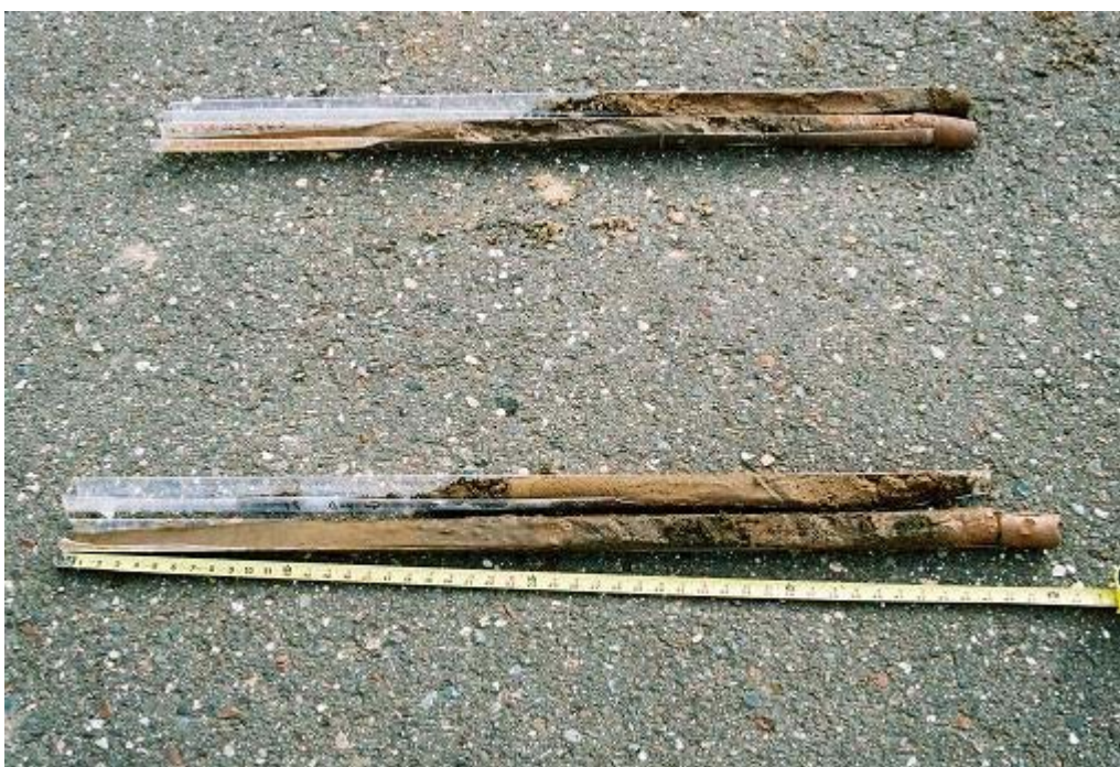
Photograph 28: 5/18/06 09:05 Soil cores at bottom of photograph from WGP-15. Shallower soils are at the top left, the bottom of the boring is at the bottom right. Photo by J. Chrestensen
