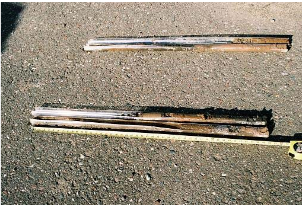
Photograph 24: 5/17/06 18:35 Soil cores at bottom of photograph from WGP-10. Shallower soils are at the top left, the bottom of the boring is at the bottom right. Note the sheen from 6.5 to 7 feet as detailed in Photograph 23. Photo by J. Chrestensen
