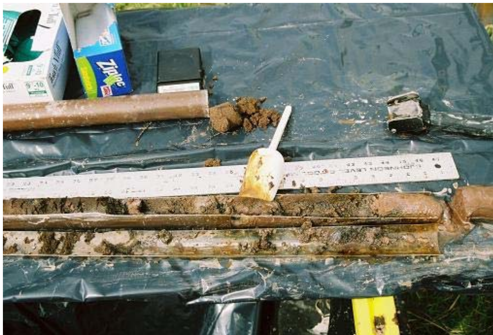
Photograph 37: 5/18/06 10:50 Detail of 6 to 8 foot interval in soil core from WGP-16 after collecting a laboratory sample. Photo by J. Chrestensen
