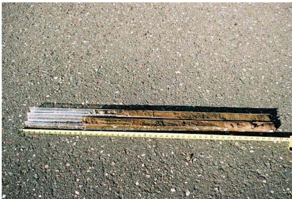
Photograph 25: 5/17/06 18:50 Soil cores from WGP-11. Shallower soils are at the top left, the bottom of the boring is at the bottom right. Photo by J. Chrestensen
