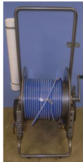
Air – Water Lines for Bladder Pump
