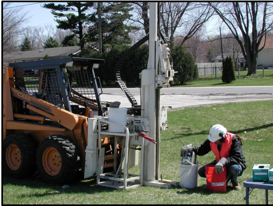
Collecting Ground Water Samples Using GeoProbe® 540B
