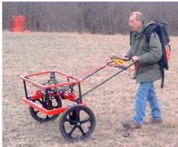
EM61: Operator pushing antennas and wearing a backpack with electronics and battery. Data are collected by a data logger mounted on handle bars.
