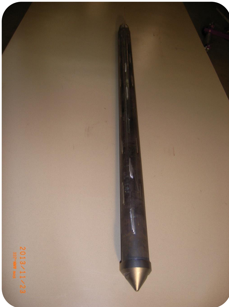
Mill Slot Probe Rod for GW Sampling
