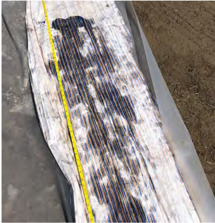
Large indication of NAPL from RW-104 (73-78 ft bgs) on NAPL FLUTe
