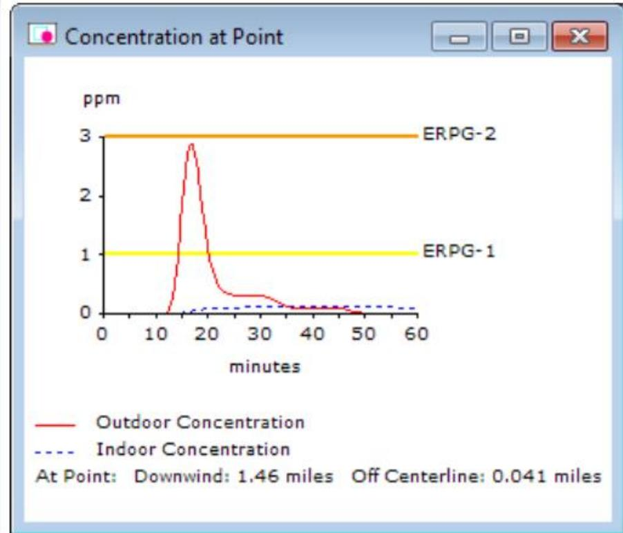
Some sample ALOHA output. On the left, the circular thermal radiation threat zone estimates for a BLEVE. On the right, a threat point graph shows the toxic concentration hazard over time at a specific location; the horizontal lines show how the concentration compares to the chosen toxic levels of concern.
