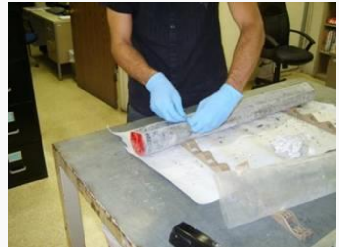
Preserving core using liquid nitrogen
