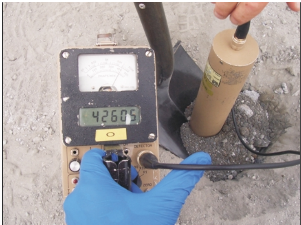
Photo 10: Gamma screening at sampling locations in the Waste Disposal Area. Background readings range from 7,000 to 14,000 counts per minute. Photo by B. Castellana taken on 06-21-06.
