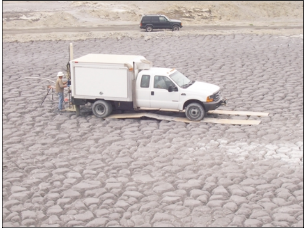
Photo 11: The EPA GeoProbe collecting waste samples in the WMU. The Geoprobe had to be driven on 1.25" plywood boards to keep it from sinking into the waste pile. Photo by B. Castellana taken on 06-27-06.
