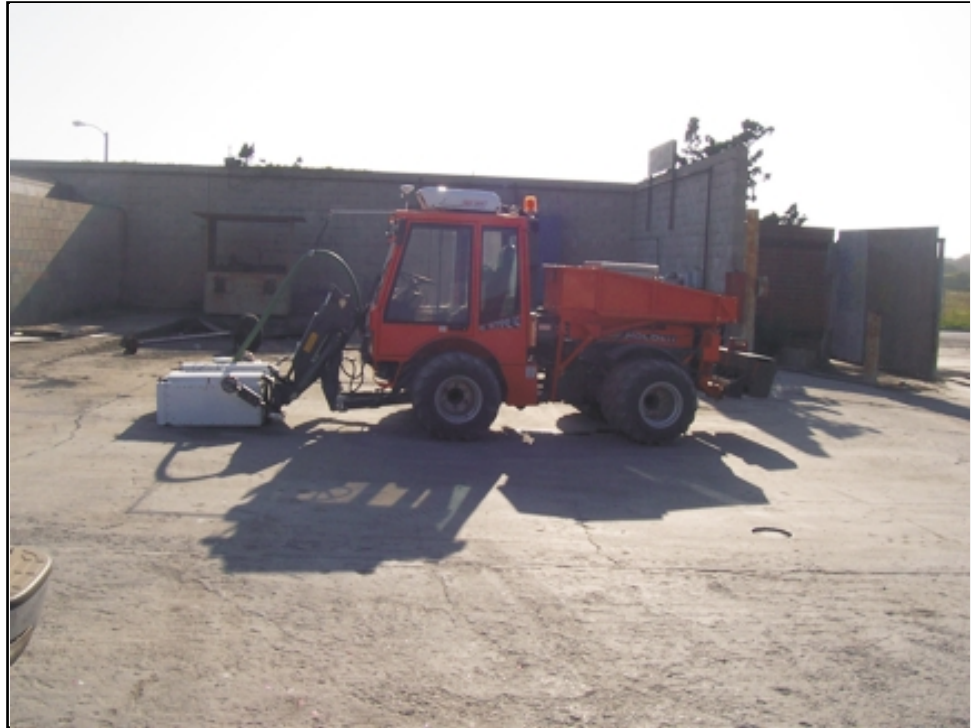
Photo 9: One method of gamma radiation screening involved the Office of Indoor Air and Radiation's tractor-mounted gamma detector - a 12x12" sodium iodide detector. Photo by B. Castellana taken on 06-21-06.
