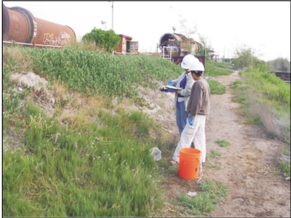
Photo 3: Collecting soil samples from the Smelter Area, along the OID. Some of the highest Gamma readings were observed in this area. Photo by B. Castellana.
