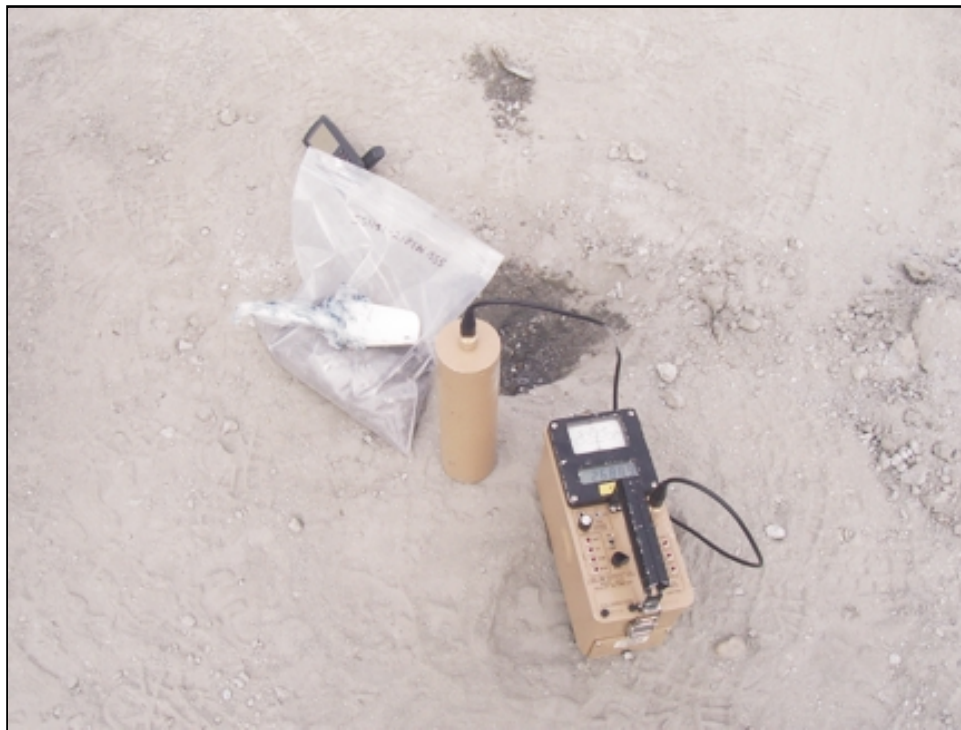
Photo 5: Collecting sample SSN51 from the Waste Disposal Area. The soil here is dominated by two to five feet of waste material used to fill in the surface. Photo by B. Castellana on 06-21-06.
