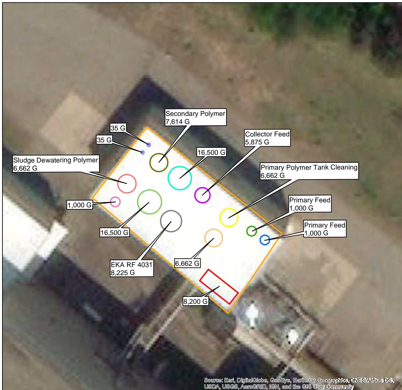
Figure 3 Tank and Drum Locations in the Chemical Storage Building East Millinocket Paper Mill Site 50 Main Street East Millinocket, Maine
