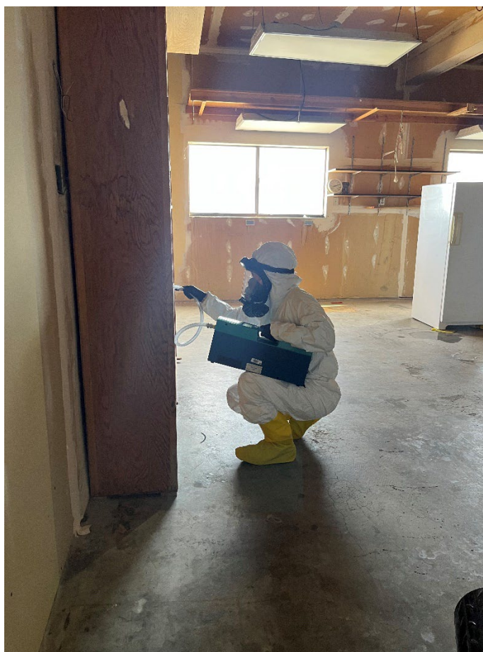
Conducting detailed air monitoring sweep in garage.
