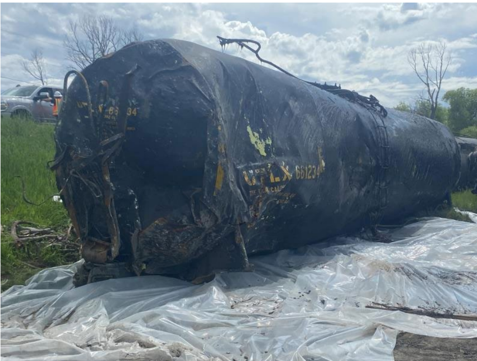
Liquid asphalt petroleum railcar moved into secondary containment.
