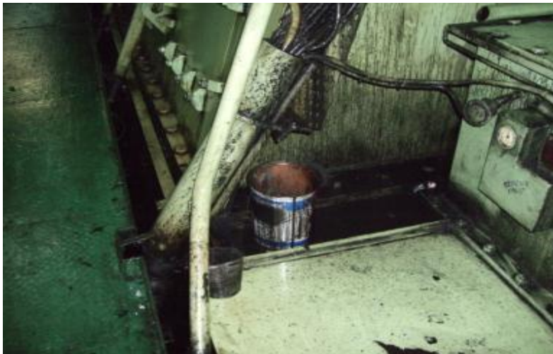
Forward starboard side of engine crankcase leaking oil
