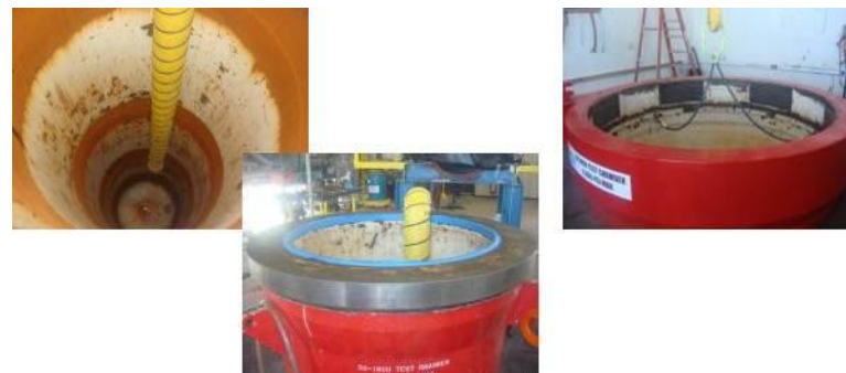
SwRI Deep Ocean Simulators (left: 7.3 m x 1.3 m \Phi , 13,500' pressure & right: 2.3 m x 5.8 m \Phi , 9,000' pressure)
