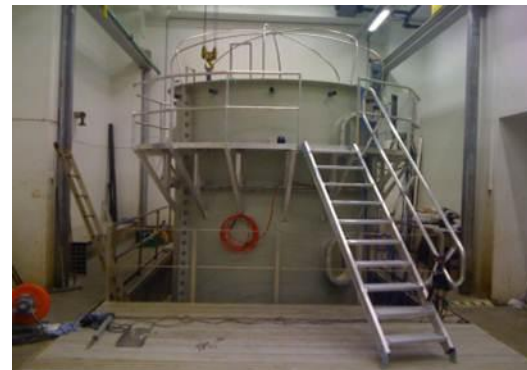
Sintef tank facility for examining subsea releases (6 m x 3 m \Phi , no pressure).
